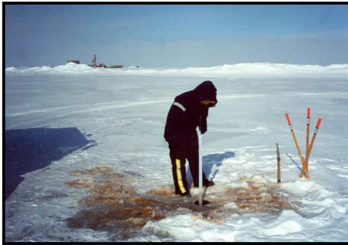
Left: Sampling at M9915 during April. Sampling methods included using a plastic bailer to collect a grab sample.
