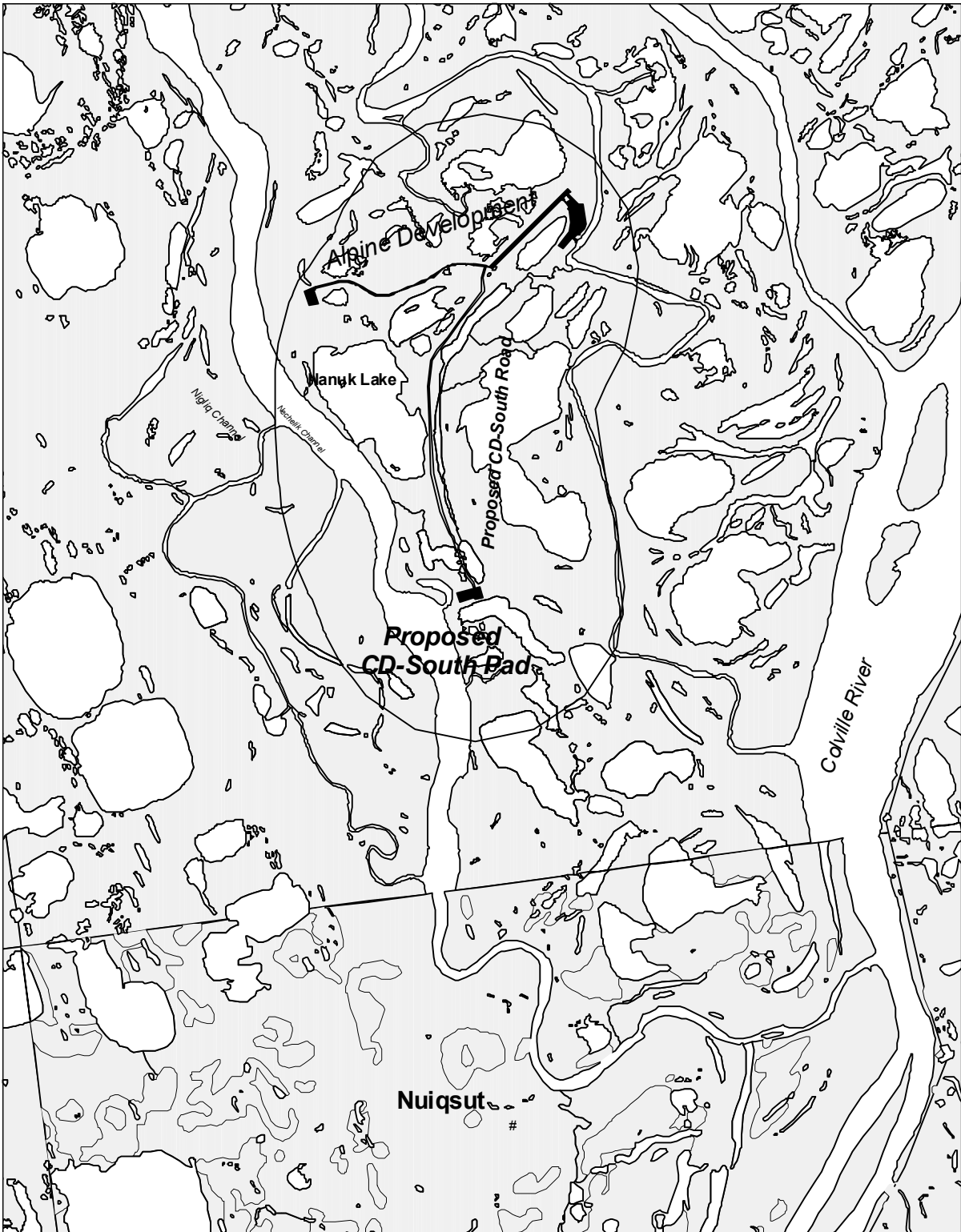
Figure 1. CD-South study area showing proposed CD-South road and facilities pad in relation to Nuiqsut and Alpine facilities (approximate boundary of study area indicated by enclosure).
