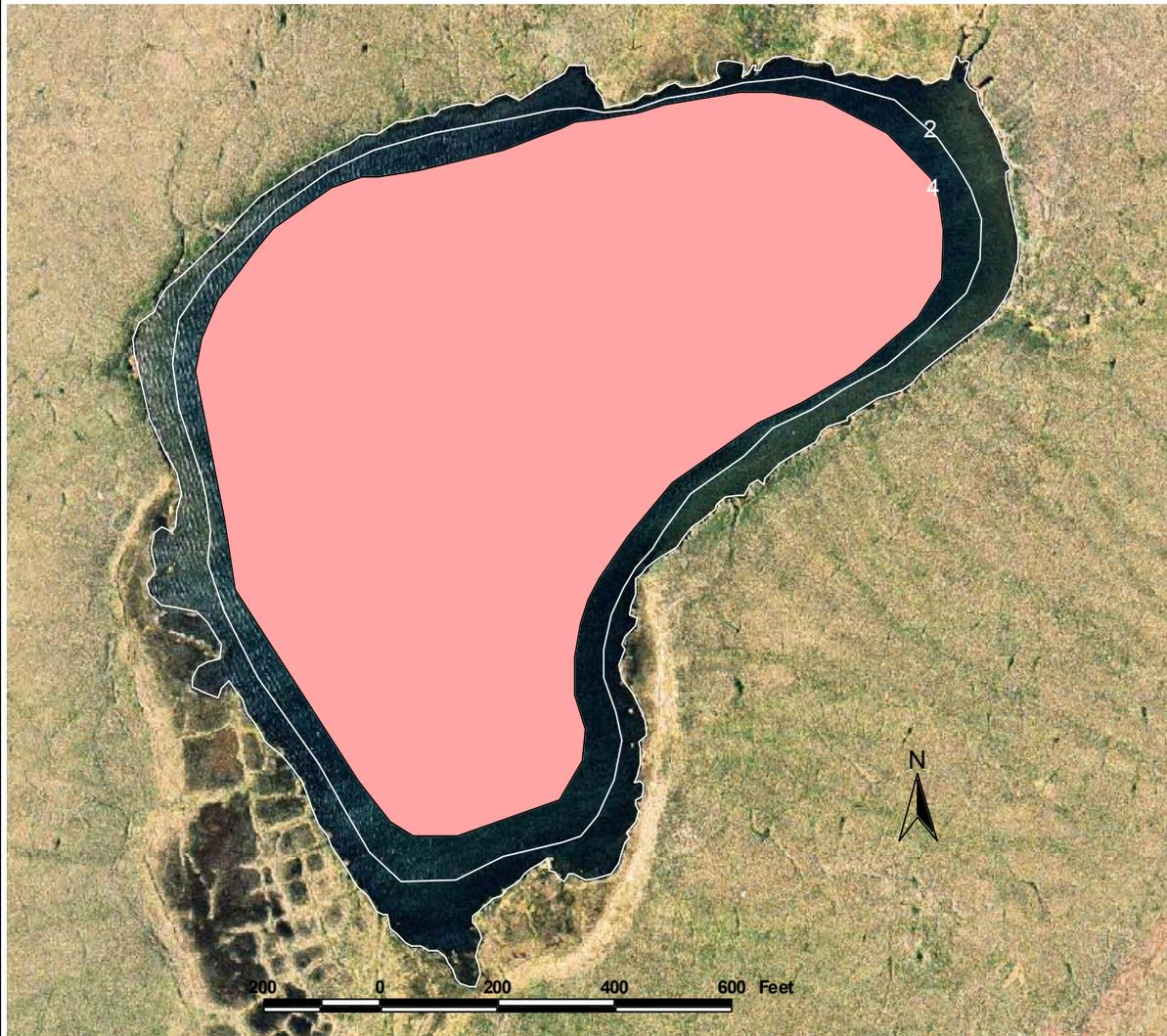
Shaded region of lake M0254 deeper than 4 ft (shaded), remainder of lake likely to be available for ice chips, based on transects surveyed on Sep. 5, 2002.
