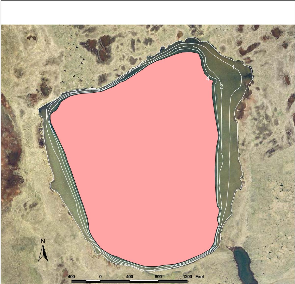
Shaded region of lake M0024 deeper than 4 ft (shaded), remainder of lake likely to be available for ice chips, based on transects surveyed on Sep. 2, 2002.
