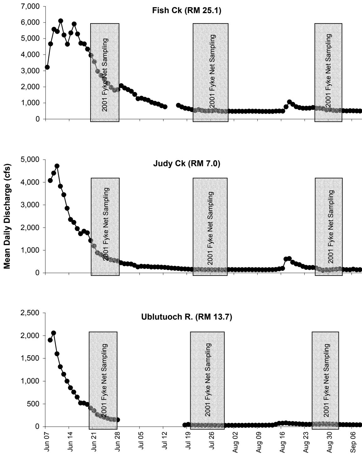
Figure 3. Discharge patterns in creeks sampled in eastern NPR-A during 2001, shaded bars indicate fyke net sampling periods (discharges from Dietzmann and Aldrich 2001, note change of scale between streams).
