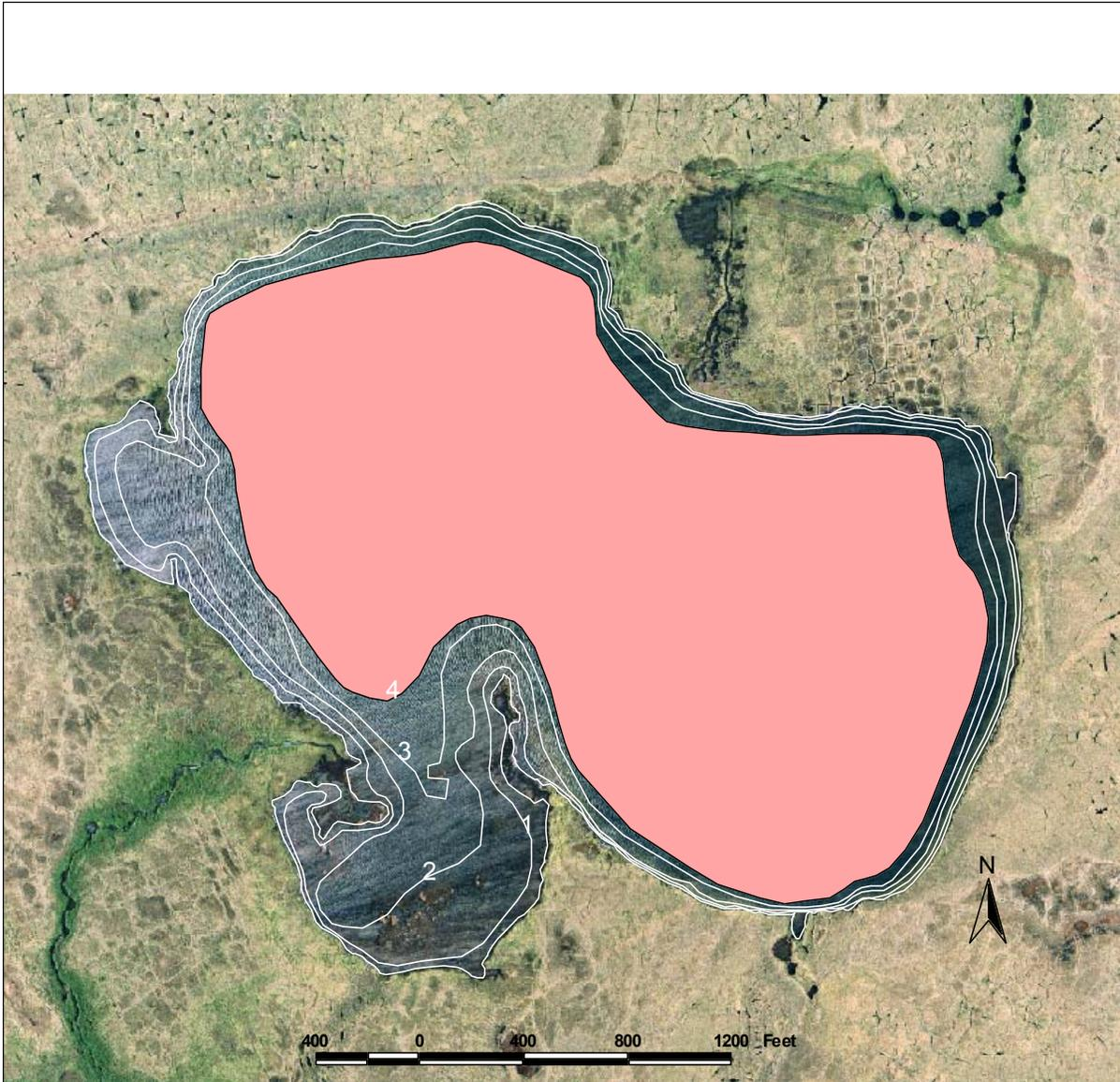
Shaded region of lake M9914 deeper than 4 ft (shaded), remainder of lake likely to be available for ice chips, based on transects surveyed on Sep. 2, 2002.
