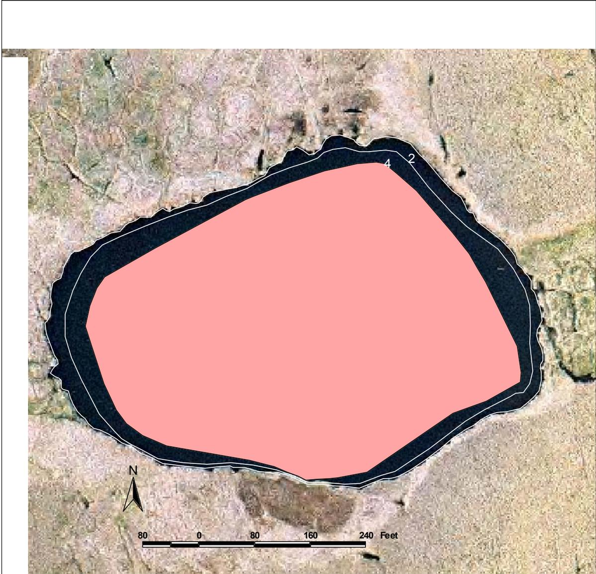
Shaded region of lake L9823 deeper than 4 ft (shaded), remainder of lake likely to be available for ice chips, based on transects surveyed on Sep. 4, 2002.
