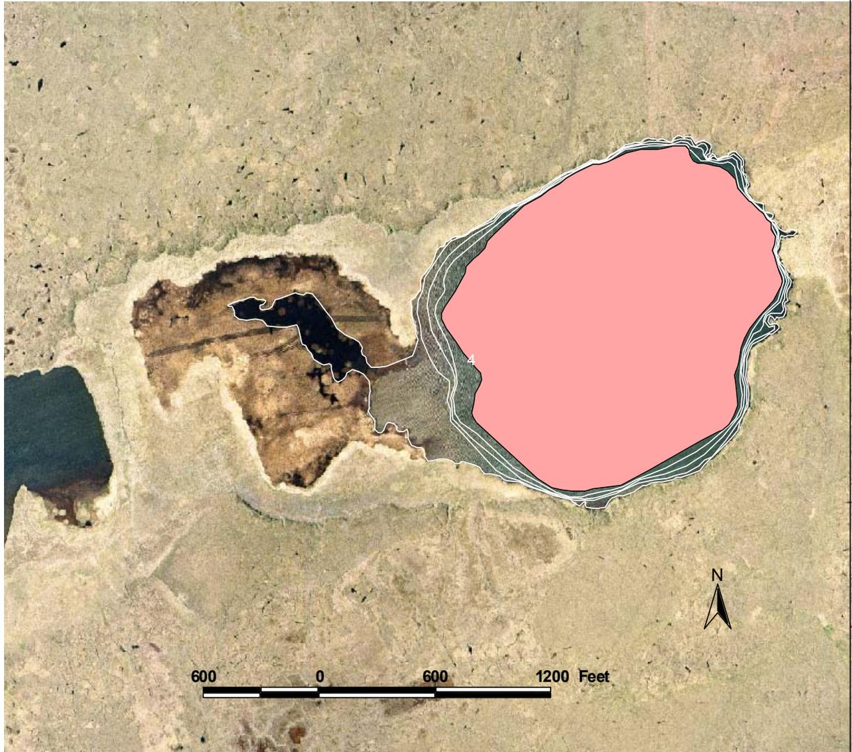
Shaded region of lake L9817 deeper than 4 ft (shaded), remainder of lake likely to be available for ice chips, based on transects surveyed on Sep 3, 2002.
