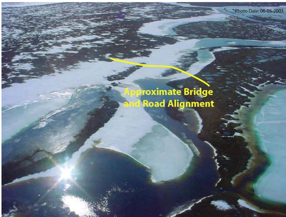
Photo 4-3 Arrival of the breakup melting front at the Ublutuoch River RM 6.8 monitoring site and proposed bridge location on 5 June at roughly 9:50 a.m. View looking southeast and upstream
