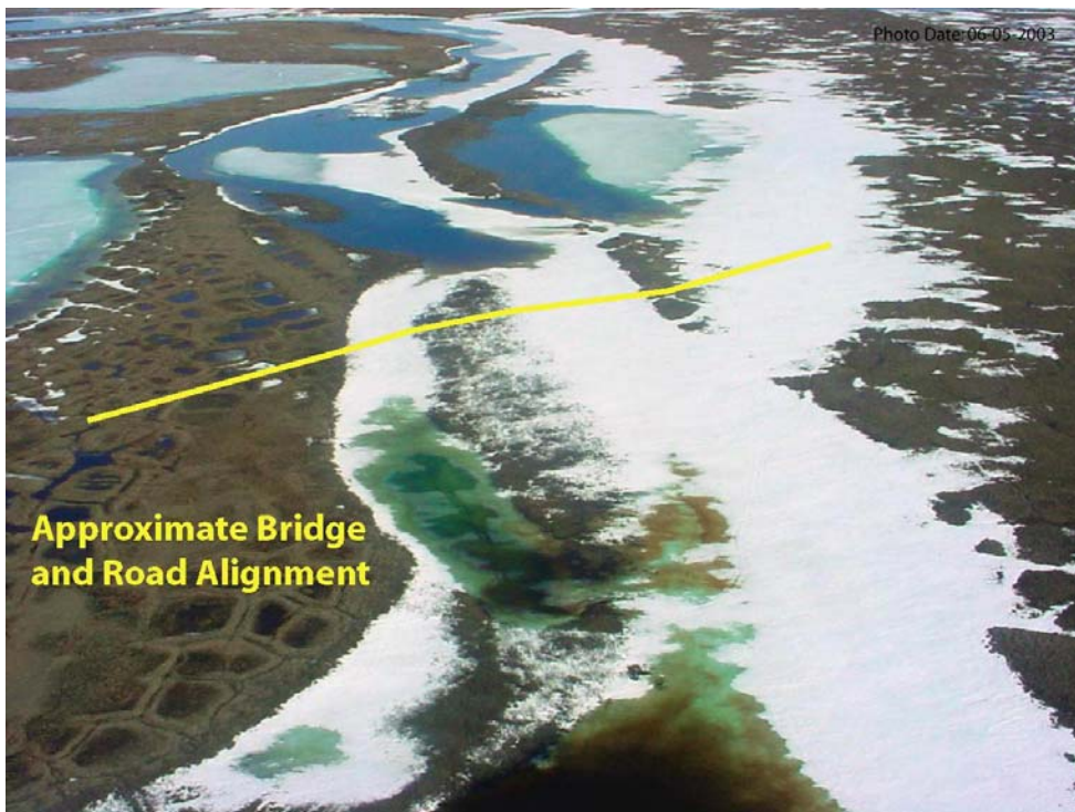
Photo 4-5 Arrival of the breakup melting front at the Ublutuoch River RM 6.8 monitoring site and proposed bridge location on 5 June at roughly 9:50 a.m. View looking northwest and downstream.
