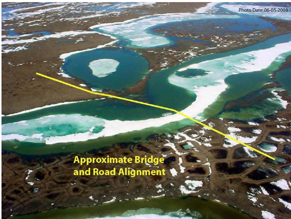
Photo 4-7 Ublutuoch River RM 1.9 monitoring site and proposed bridge location on 5 June prior to the arrival of breakup flows. Water in channel and nearby lake basins is from local melt and influx from minor tributaries. View looking northwest.
