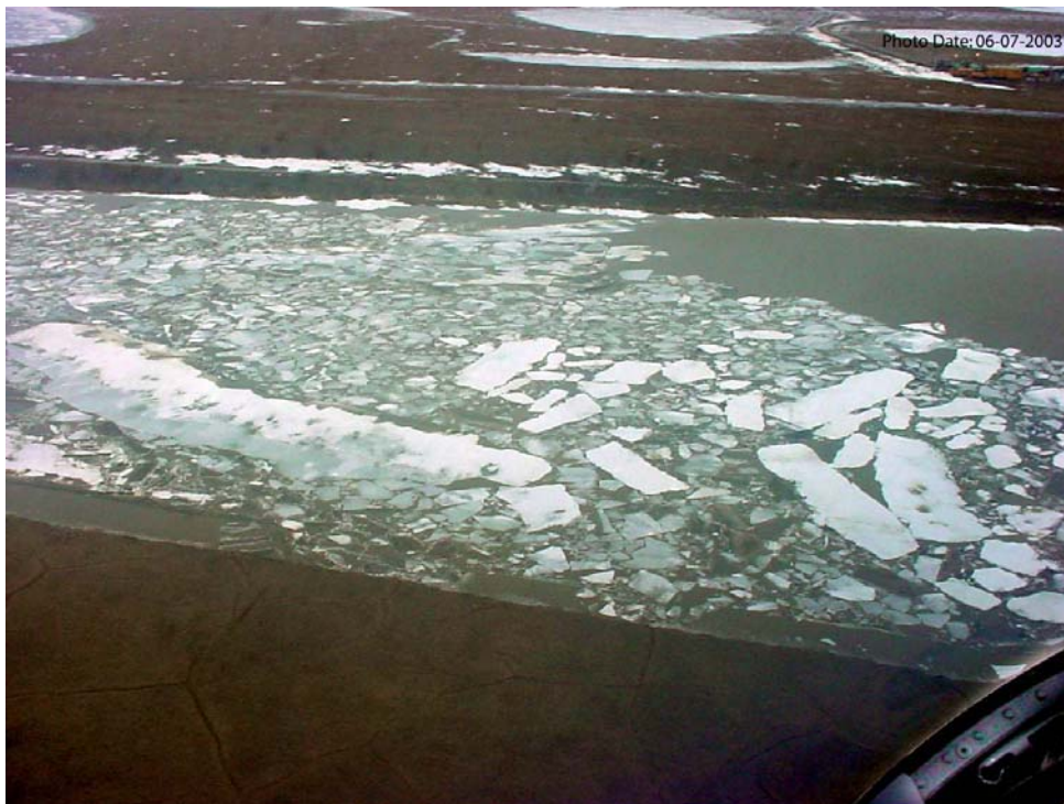
Photo 3-2 Breakup conditions on the Nigliq Channel near the proposed bridge crossing site on 7 June. Conditions shown are several hours prior to the occurrence of the breakup peak water surface elevation in the channel. View looking west. CD-2 is in upper right corner of photo. Flow is from right to left.
