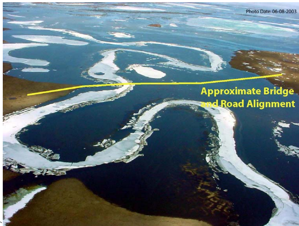
Photo 4-7 Ublutuoch River RM 1.9 monitoring site and proposed bridge location on 5 June prior to the arrival of breakup flows. Water in channel and nearby lake basins is from local melt and influx from minor tributaries. View looking northwest.
