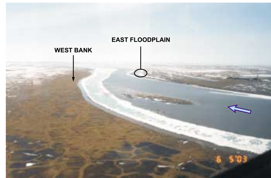
6. Extent of winter ice is indicative of main low flow channel as shown in Airphoto Figure 1.
