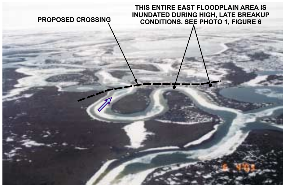
1. Long range view illustrating the sharp meander bends.
