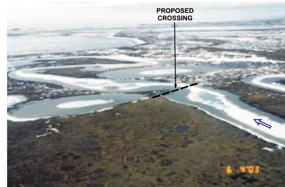
3. Width of ice is indicative of the width and location of the winter low flow channel. At the crossing, maximum velocities and bank erosion potential expected to occur along the right (east) bank.
