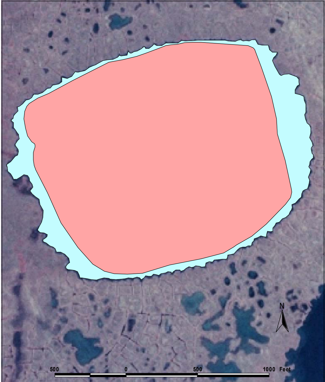
Regions of lake M0533 less than 4 feet deep (light-shaded) and likely to available for ice chips, based on transects surveyed on July 24, 2005.
