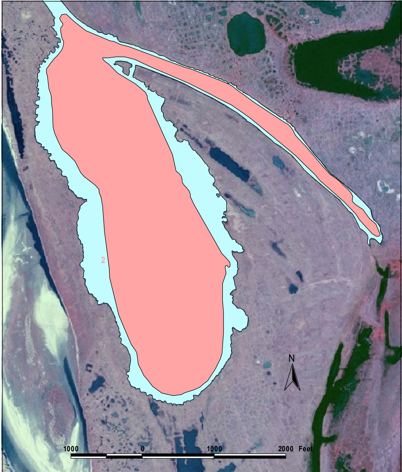
Regions of lake M0517 less than 4 feet deep (light-shaded) and likely to be available for ice chips, based on transects surveyed on July 23, 2005.
