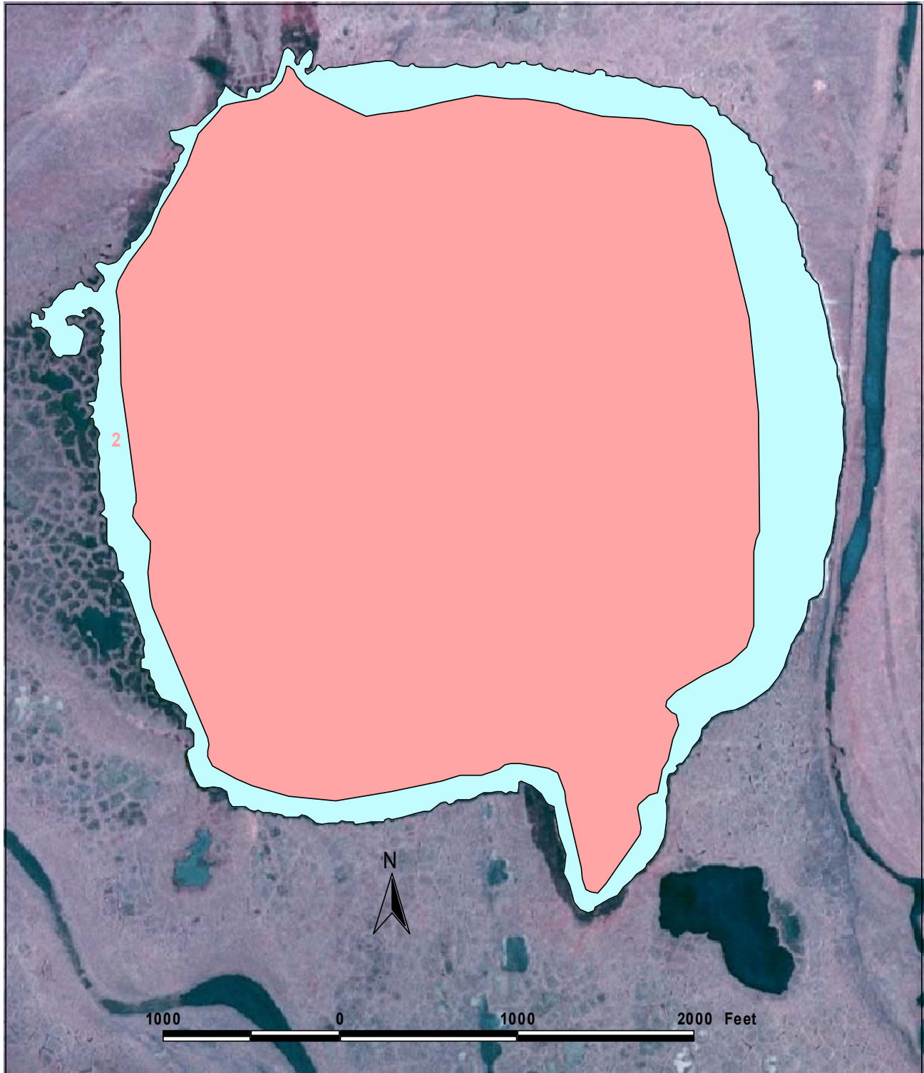
Regions of lake B84140 less than 4 feet deep (light-shaded) and likely to be available for ice chips, based on transects surveyed on July 22, 2005.
