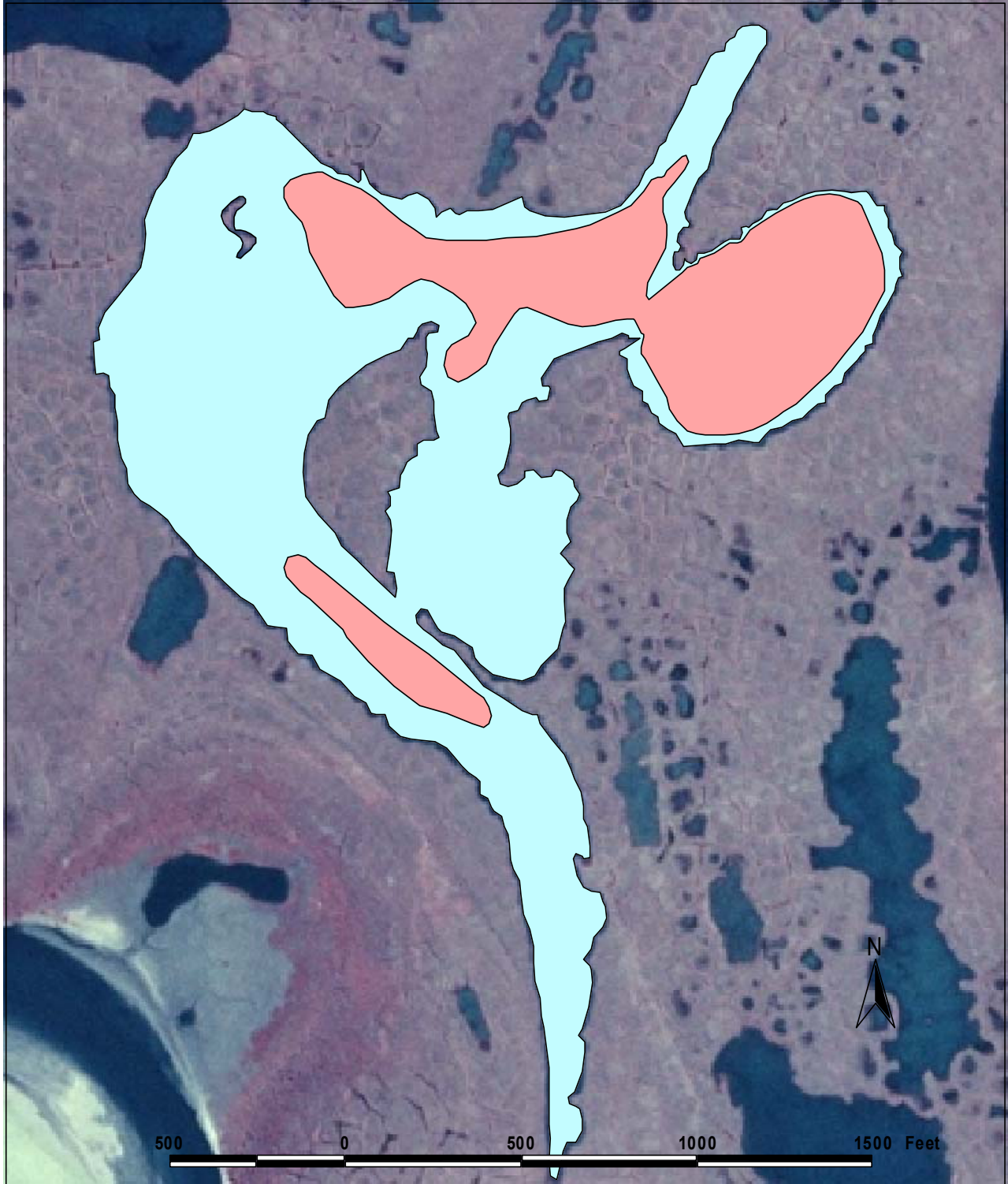
Regions of lake M0532 less than 4 feet deep (light-shaded) and likely to be available for ice chips, based on transects surveyed on July 24, 2005.
