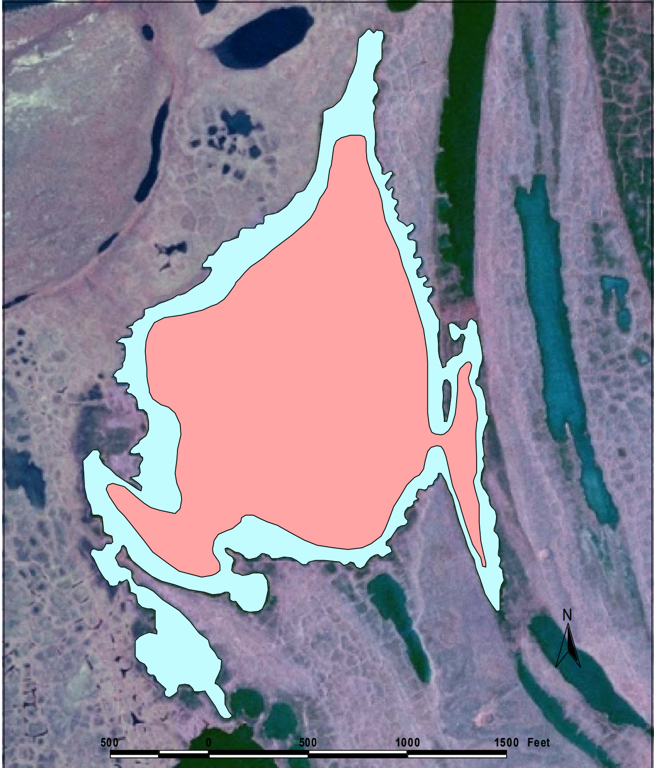
Regions of lake M0531 less than 4 feet deep (light-shaded) and likely to be available for ice chips, based on transects surveyed on July 24, 2005.
