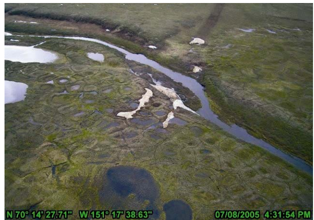
Photo 5-28 Ublutuoch River Ice Bridge after breakup with the ice road remnants still in place, July 8, 2005
