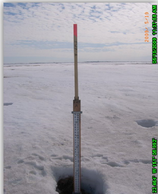
PHOTO 3.1: STAFF GAGE INSTALLED AT SITE FWP, MAY 19, 2009
