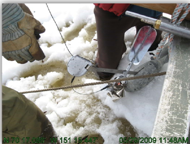
PHOTO 3.2: UBLUTUOCH RIVER BOAT DISCHARGE MEASUREMENT INSTRUMENTATION, MAY 29, 2009
