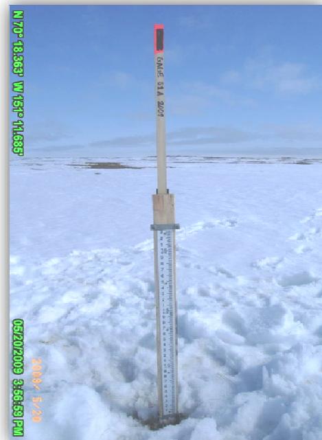
PHOTO 3.1: STAFF GAGE INSTALLED AT SITE S1, MAY 20, 2009
