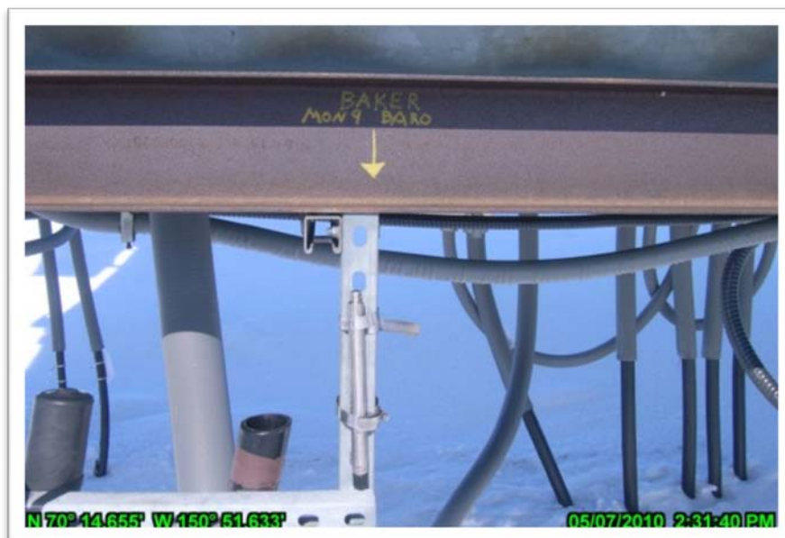
Photo 3.5: BaroTroll® atmospheric pressure sensor installed at MON9; May 7, 2010.
