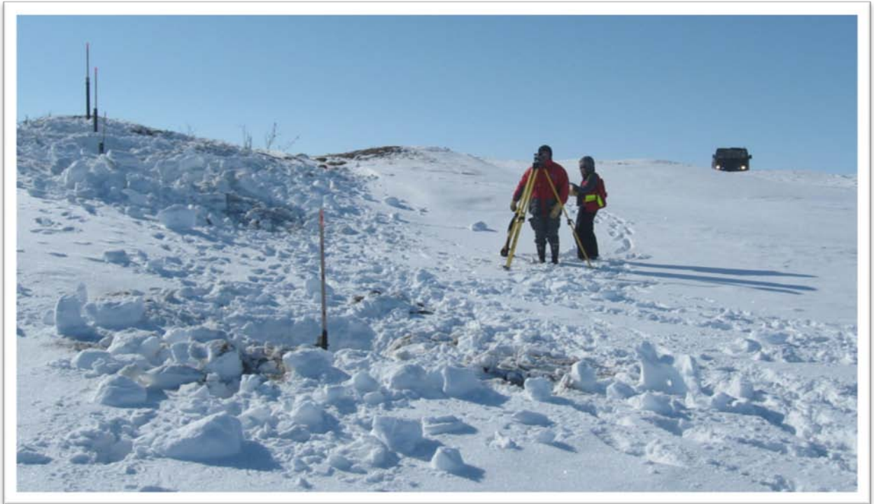
Photo 3.3: Surveying MON9 (HDD) gages; gage B in foreground, gages C, D, and E in background; May 7, 2010.
