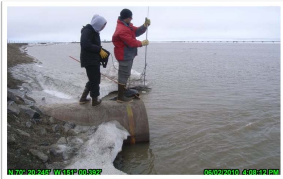
Photo 3.7: Culvert velocity measurement using USGS wading rod on upstream side of culvert CD2-15, looking west; June 2, 2010.
