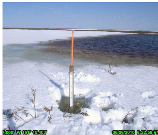
Photo 3.1: Staff Gage Installed at UB6.9-A, June 6, 2010
