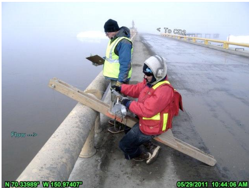
PHOTO 5.9: DISCHARGE MEASUREMENT AT THE 452-FOOT SWALE BRIDGE; MAY 29, 2011
