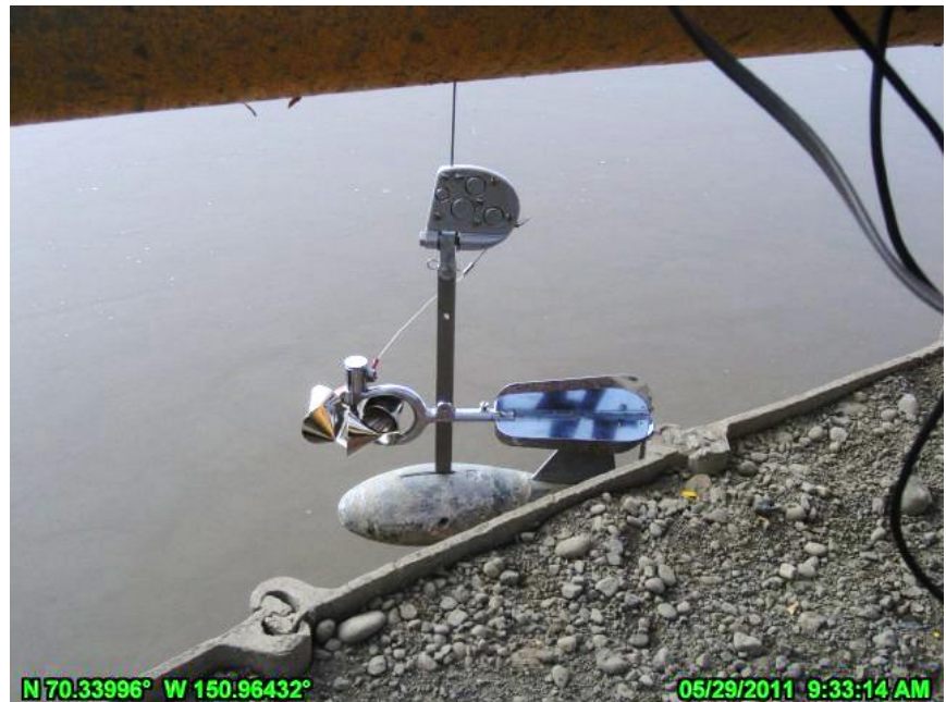
PHOTO 3.4: PRICE AA VELOCITY METER AND 30-POUND COLUMBUS-TYPE SOUNDING WEIGHT; MAY 29, 2011
