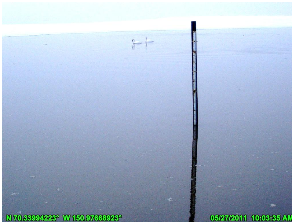
PHOTO 3.2: PERMANENT DIRECT-READ STAFF GAGE G3 NEAR CD2 ROAD SWALE BRIDGES; MAY 27, 2011
