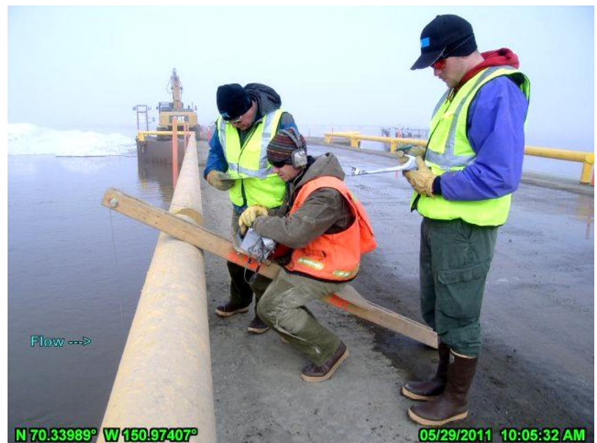
PHOTO 3.5: PERFORMING A DISCHARGE MEASUREMENT ON THE UPSTREAM (SOUTH) SIDE OF THE LONG SWALE BRIDGE USING A PRICE AA VELOCITY METER AND SOUNDING REEL MOUNTED ON A BOOM; MAY 29, 2011
