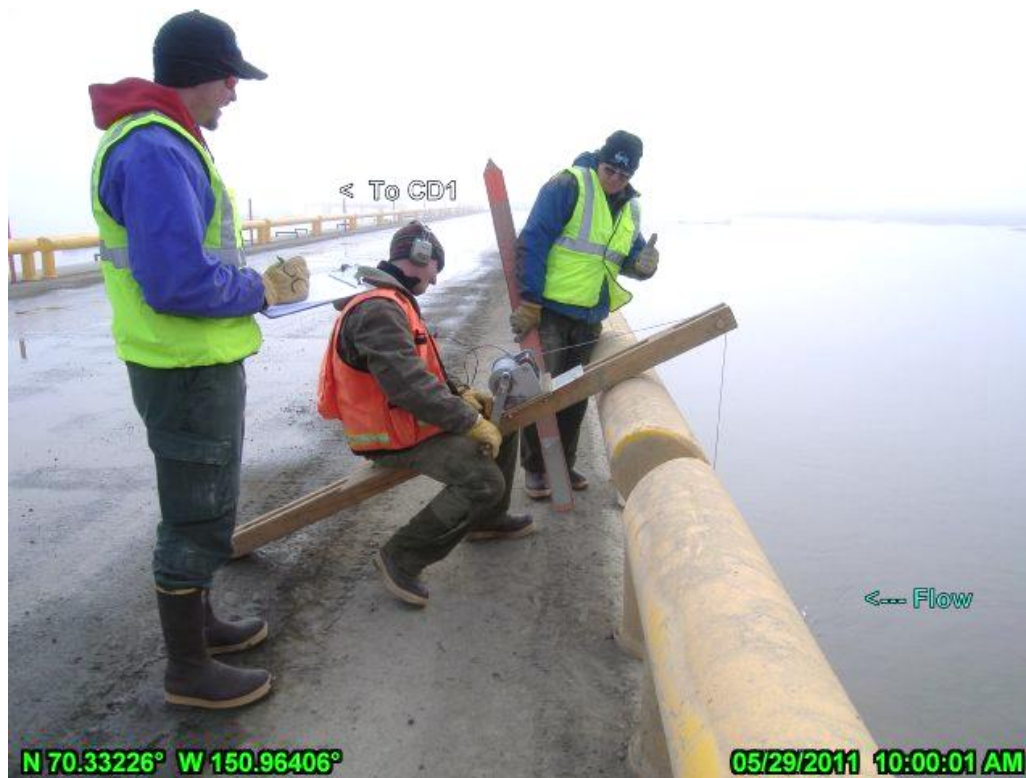
PHOTO 4.68: DISCHARGE MEASUREMENT FROM THE 452-FOOT SWALE BRIDGE, LOOKING EAST; MAY 29, 2011
