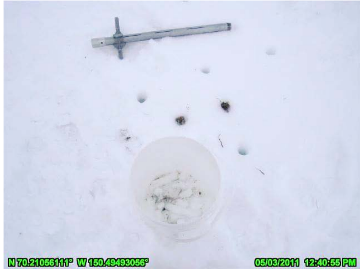
PHOTO 3.3: MODEL 3600 MT. ROSE SNOW SAMPLER (TOP) AND BUCKET FOR POOLED SNOW SAMPLES (BOTTOM) WITH SAMPLE HOLES
