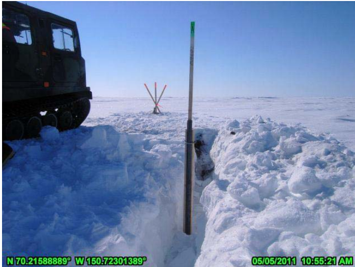
PHOTO 3.2: NEWLY ESTABLISHED TBM (BACKGROUND) AT LAKE M9602 AND GAGE M9602- A (FOREGROUND), PRE- BREAKUP
