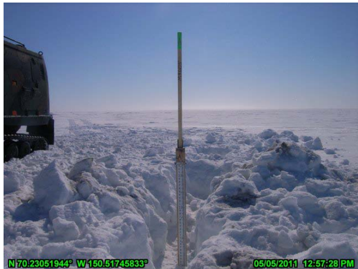
PHOTO 3.1: HYDROLOGIC GAGE AT LAKE M9605, PRE-BREAKUP
