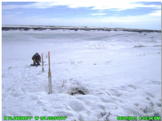
Photo 3.1: Staff gage setup at a site along the Ublutuoch River, looking south; May 21, 2011
