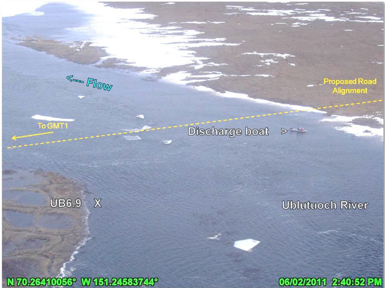
Photo 4.60: Baker crew performing discharge measurement at the proposed Ublutuoch bridge location (UB6.8), looking downstream (northeast); June 2, 2011
