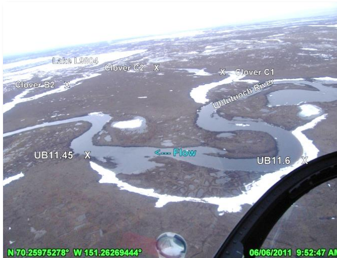
Photo 4.50: Flow confined to channel banks as stage drops at UB11.45-UB11.6, looking south; June 6, 2011
