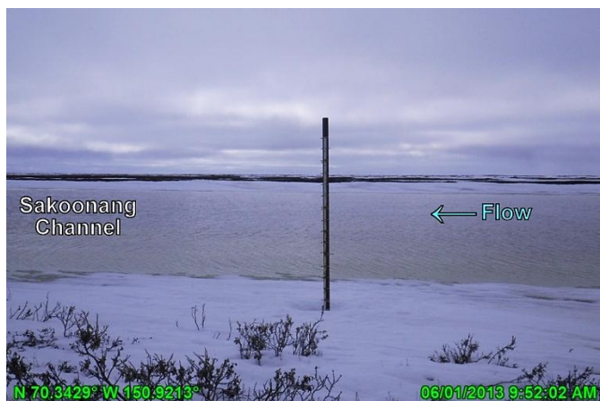
Photo 2.3: Permanent, direct-read staff gage near CD1; June 1, 2013
