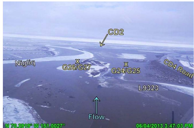
Photo 3.58: Overbank flooding at the proposed Lake L9323 and Nigliq Channel crossing, looking north; June 4, 2013
