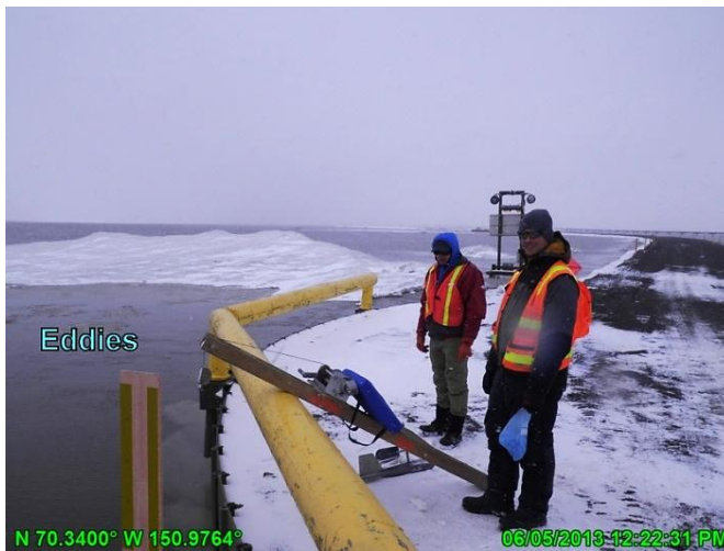
Photo 3.33: Beginning direct discharge measurements at the long swale bridge with snow berm upstream of left bank, looking southwest; June 5 2013
