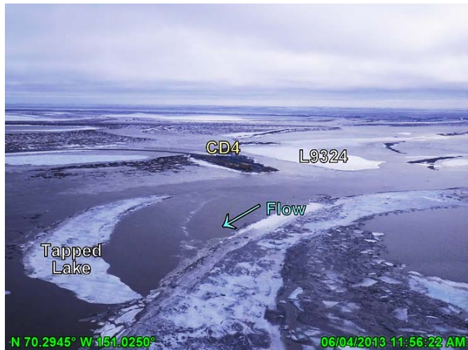
Photo 3.11: CD4 with diverted floodwater around the Nigliq Channel ice jam, looking southeast; June 4, 2013
