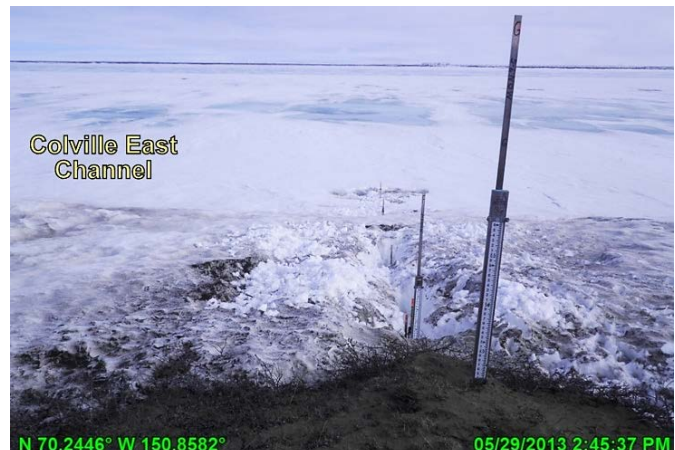
Photo 2.4: Temporary, indirect-read gage set at MON9; May 29, 2013
