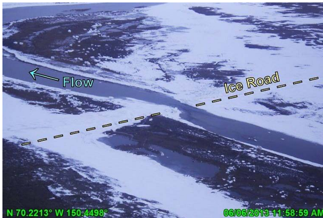
Photo 3.46: Low velocity flow passing Kachemach River ice bridge, looking north; June 6, 2013
