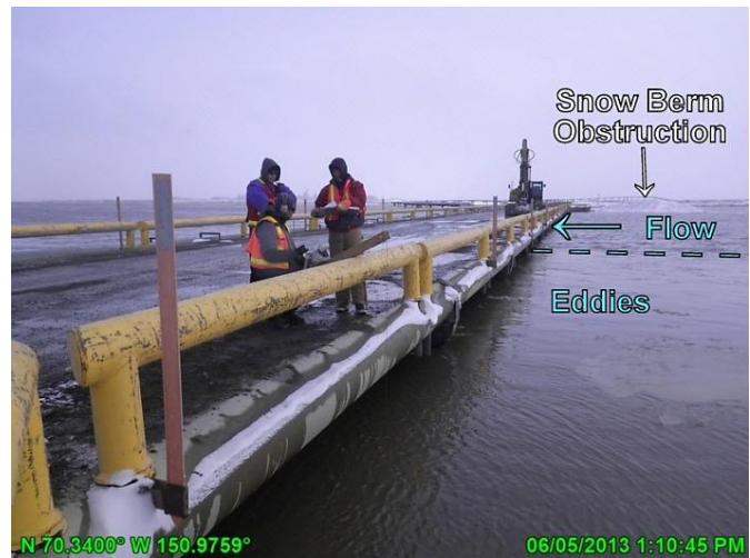
Photo 3.34: Conditions through the long swale bridge during direct discharge measurements, looking east; June 5, 2013
