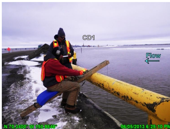
Photo 2.5: Price AA velocity meter in use at an Alpine facility bridge; June 5, 2013
