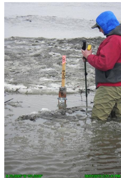
Photo 2.2: Reading the water level off a staff gage at G29; June 1, 2013
