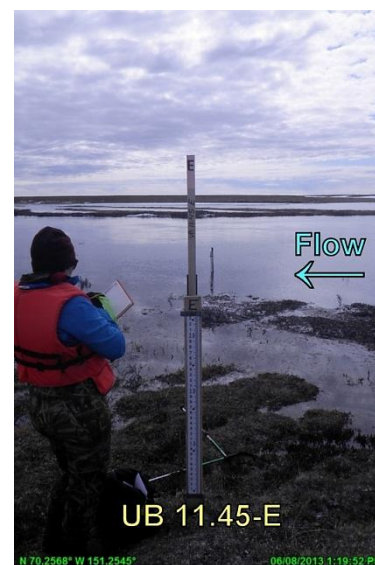
Photo 2.1: WSE reading at UB11.45, looking northeast; June 8, 2013
