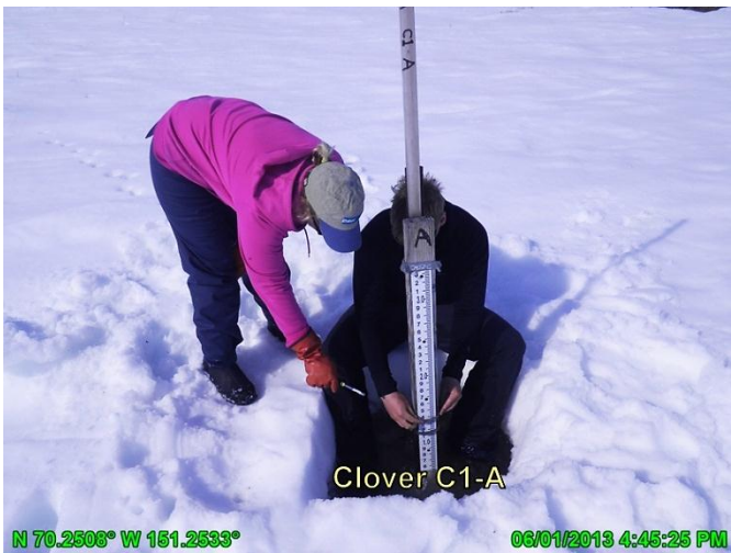
Photo 2.3: Installing a PT at Clover C1, looking northeast; June 1, 2013
