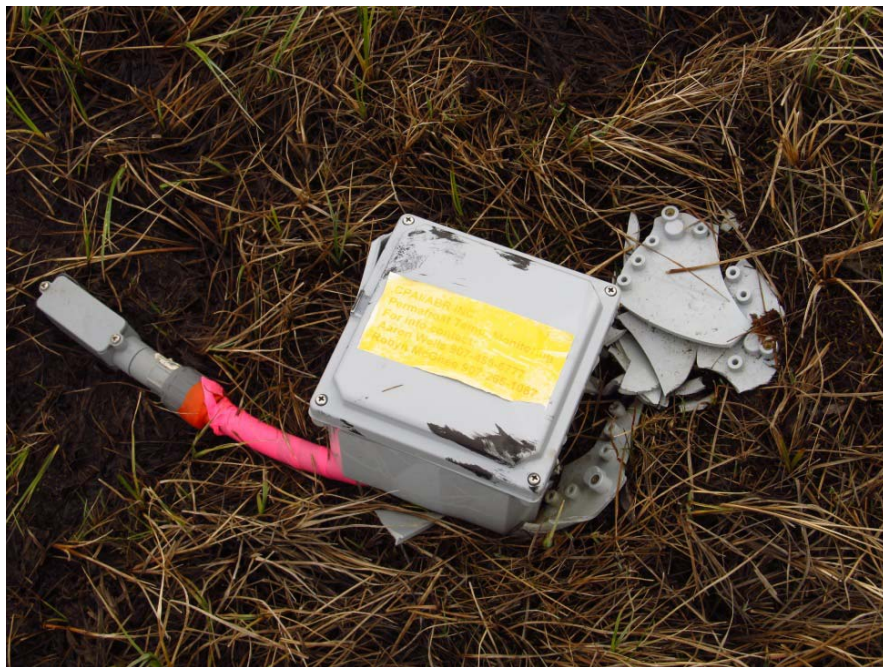
Figure 11. View of water in the bottom of a Hobo Installation box at plot rs-pc11 (above) and damage to the Hobo installation box at plot ts-pc14 caused by an ice pad (below), CD5 Habitat Monitoring Study, northern Alaska, 2013–2014.
