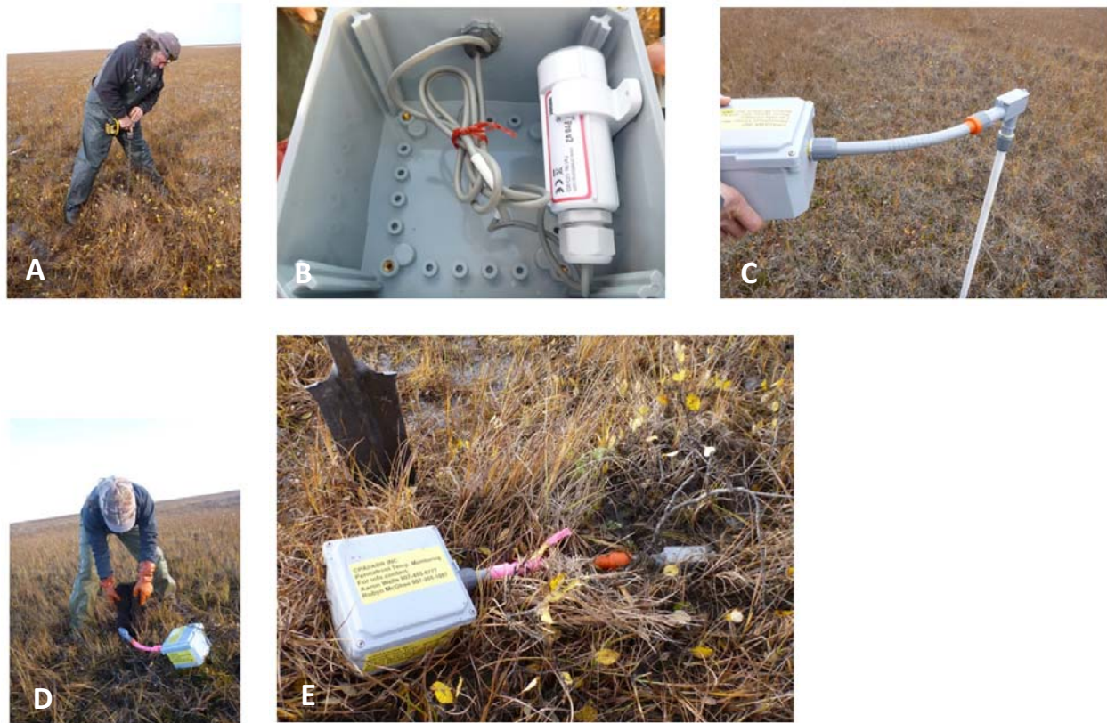
Figure 3. Temperature Logger installation and field deployment, CD5 Habitat Monitoring Study Area, northern Alaska, 2013–2014. Installation includes a) drilling a 1-m deep hole with a power drill; b) feeding the HOBO logger cables through the water proof box and into the PVC tube to a depth of 11.8 in (30 cm) and 39.4 in (100 cm) from the soil surface; c) sealing the box and PVC tube and reinforcing connections with waterproof tape; d) removing and restoring the surface organic mat; and e) an image of the final logger installation.
