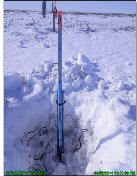
Photo 2.3: PT installed during rehabilitation of gage UB6.7-A; May 2, 2014
