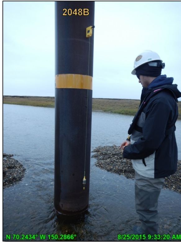
Photo A.51: Miluveach River VSM measurement with plumb bob, looking southwest; August 25, 2015
