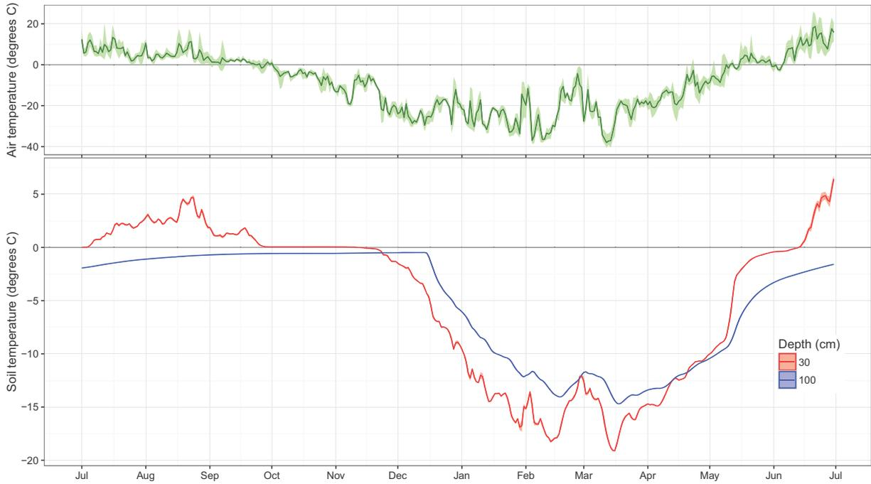
Appendix B-13. Time series of daily median soil temperature at 30 cm and 100 cm at Permafrost Monitoring Plot ts-pc08 (hobo serial number 10392129) and average daily air temperature at the Alpine weather station, CD5 Habitat Monitoring Study, northern Alaska, July 2014–June 2015.
