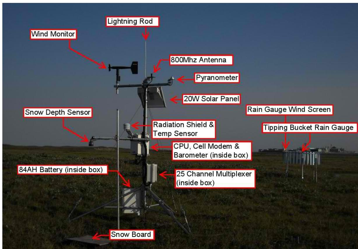
Figure 3. Annotated photograph of the Alpine Weather Station illustrating the station layout and instrumentation, Colville River Delta, northern Alaska, 2013–2015.
