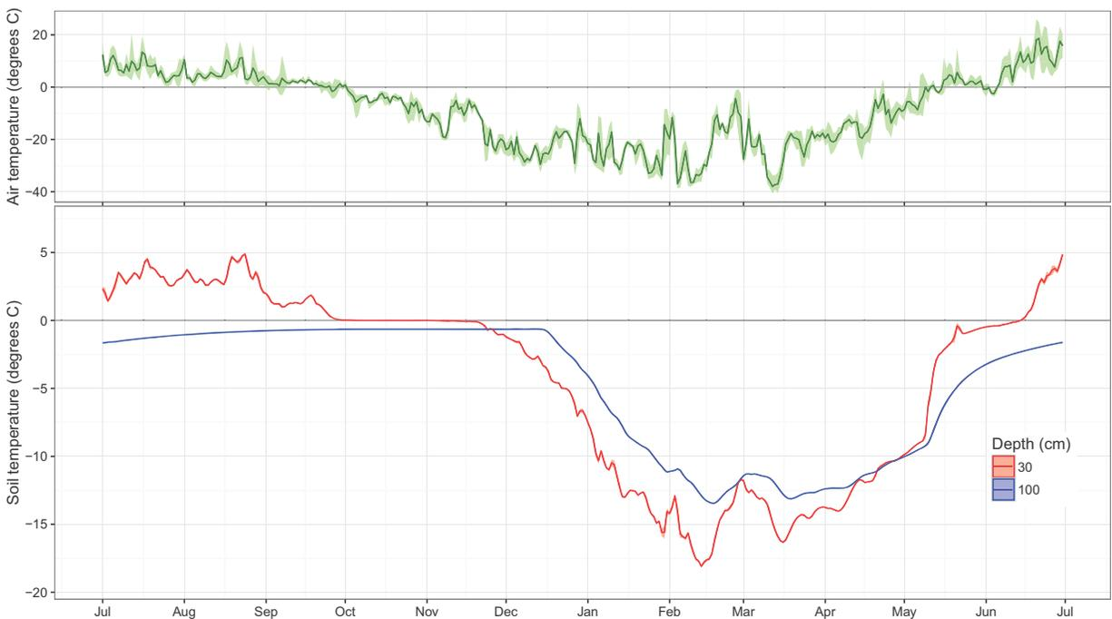
Appendix B-14. Time series of daily median soil temperature at 30 cm and 100 cm at Permafrost Monitoring Plot ts-pc12 (hobo serial number 10392133) and average daily air temperature at the Alpine weather station, CD5 Habitat Monitoring Study, northern Alaska, July 2014–June 2015.
