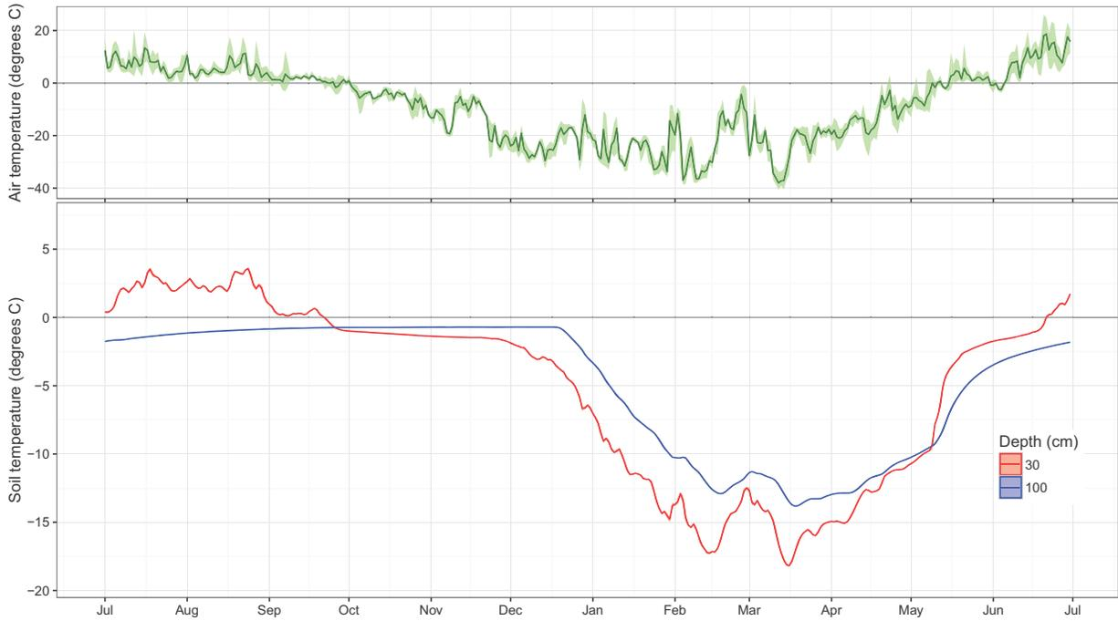
Appendix B-11. Time series of daily median soil temperature at 30 cm and 100 cm at Permafrost Monitoring Plot tn-pc15 (hobo serial number 10392136) and average daily air temperature at the Alpine weather station, CD5 Habitat Monitoring Study, northern Alaska, July 2014–June 2015.
