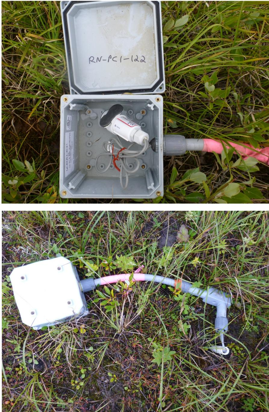
Figure 14. Photos of water in the bottom of a Hobo Installation box at RN-PC01 (top) and t-joint disconnected at plot TS-PC08 (bottom) resulting from disturbance by spring breakup flooding, CD5 Habitat Monitoring Study, northern Alaska, 2015.
