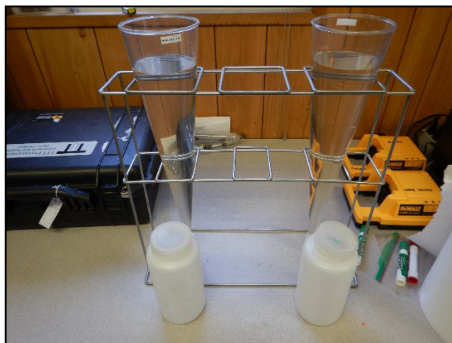
Photo 3: Volumetric Test for Settleable Solids
