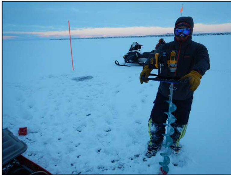
Photo 1: 6-Inch Diameter Auger with Drill
