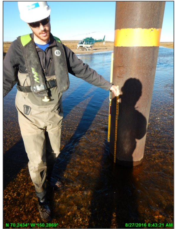
Photo A-49: Miluveach River post breakup scour measurement, looking northwest; August 27, 2016
