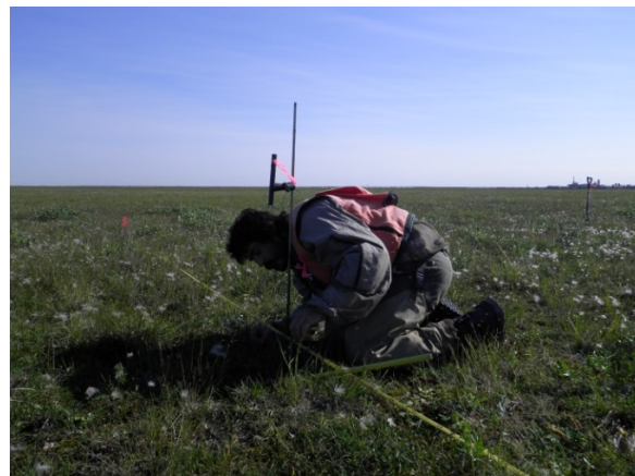
Botanist using a laser pointer mounted on a frost probe to conduct point counts along a vegetation sampling line.
