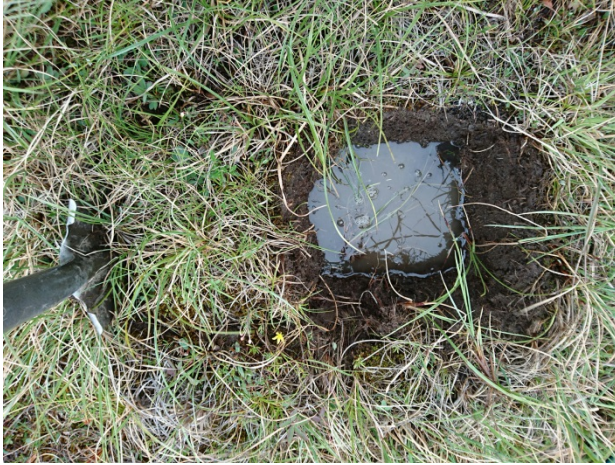
Figure 3.4. Example of a soil pit demonstrating the temporary removal of the 2013 soil plug, and the shovel slice for the 2016 soil plug, used to describe soil at vegetation plots, CD5 Habitat Monitoring Study Area, northern Alaska, 2013 and 2016.
