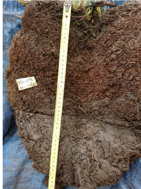
Figure 3.4. Example of a soil pit demonstrating the temporary removal of the 2013 soil plug, and the shovel slice for the 2016 soil plug, used to describe soil at vegetation plots, CD5 Habitat Monitoring Study Area, northern Alaska, 2013 and 2016.
