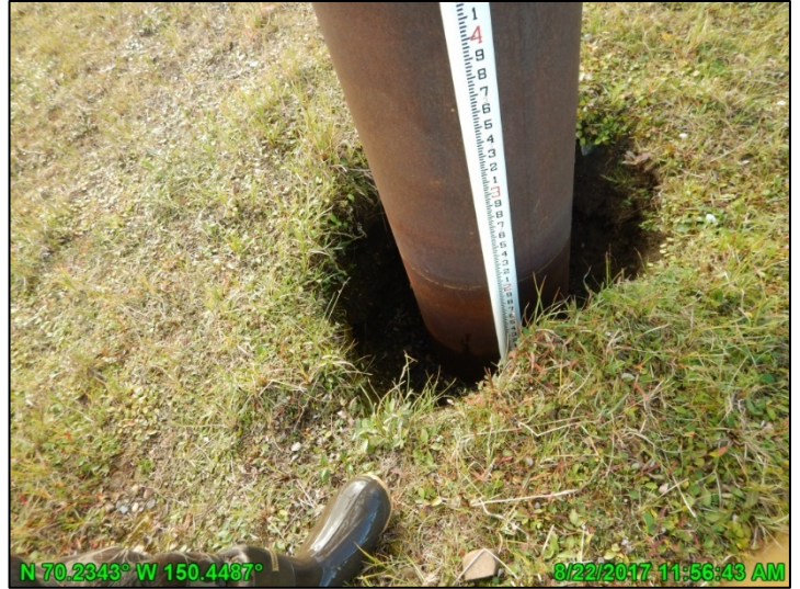
Photo A-26: Kachemach River VSM ground depression measurement; August 22, 2017
