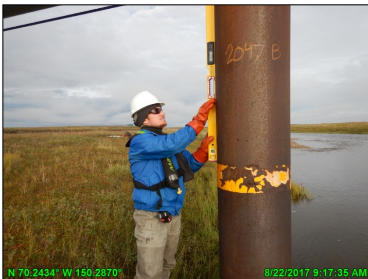
Photo A-31: Miluveach River VSM tilt measurement; August 22, 2017
