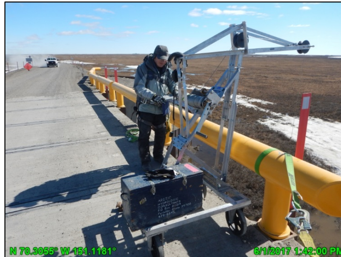
Photo 2.5: Measuring discharge at the Nigliagvik Bridge; June 1, 2017
