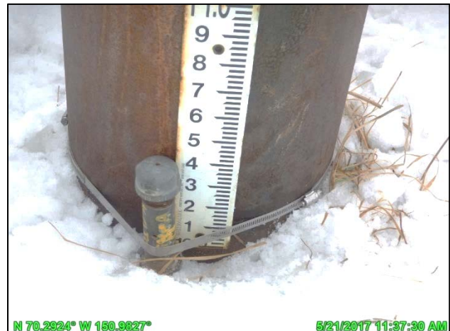
Photo 2.4: PT on direct-read gage G18-B on a VSM; May 21, 2017
