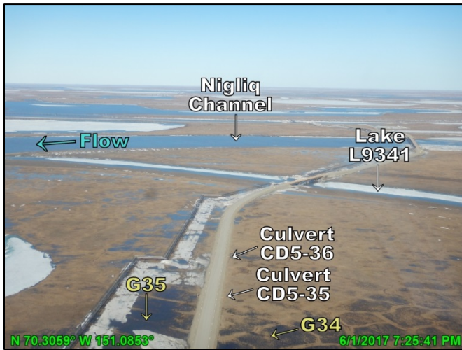
Photo 4.24: Local melt near culverts associated with gages G34/G35, looking west; June 1, 2017
