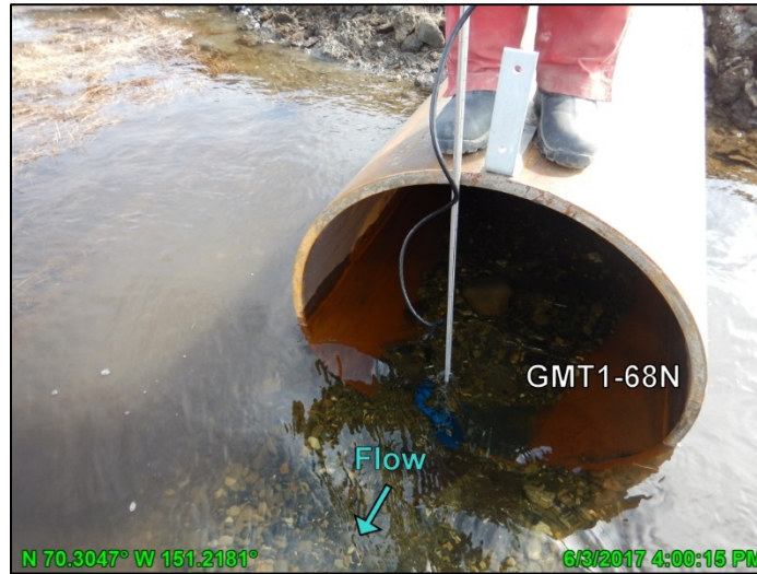
Photo 3.10: Measuring discharge at GMT1-68, looking southeast; June 3, 2017
