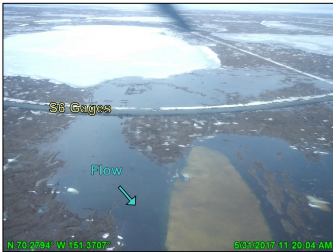
Photo 4.32: S6 gages and culverts the day of spring peak stage and discharge, looking south (upstream); May 31, 2017
