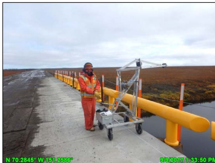
Photo 2.4: Measuring summer discharge at the Tinmiaqsiugvik Bridge; September 9, 2017
