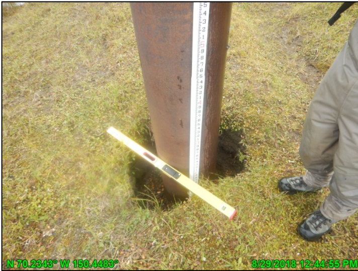
Photo A.29: Kachemach River VSM ground depression measurement; August 29, 2018
