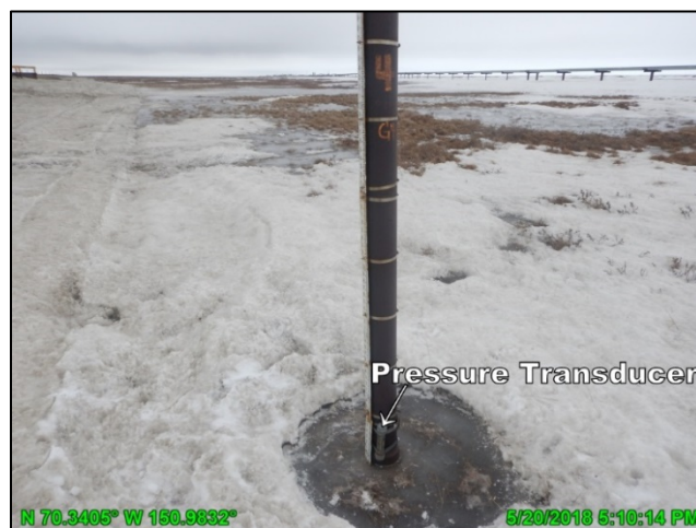
Photo 2.4: PT on direct-read gage G4; May 20, 2018
