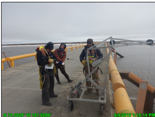
Photo 2.5: Measuring discharge at the Nigliq Bridge; June 4, 2018
