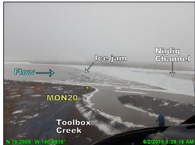
Photo 4.13: Ice jam and conditions the day prior to peak stage at MON20, looking southwest (upstream); June 2, 2018
