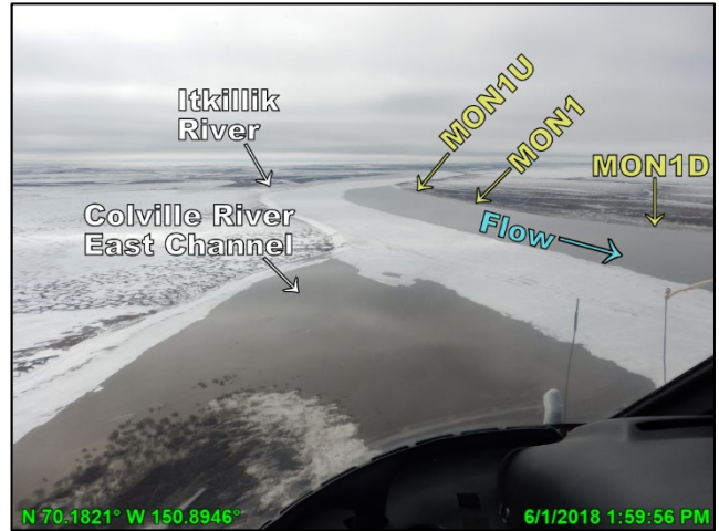
Photo 4.2: Intact channel ice through the MON1 reach the day prior to peak stage at MON1C, looking southwest (upstream); June 1, 2018
