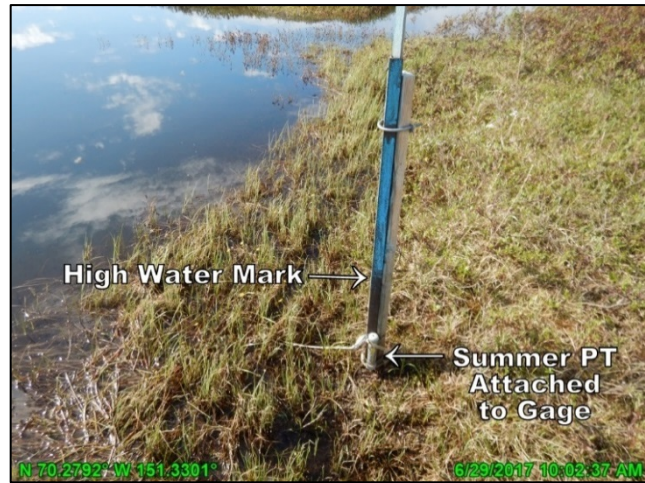
Photo 2.2: Chalked gage S5-C with HWM and PT; June 29, 2017
