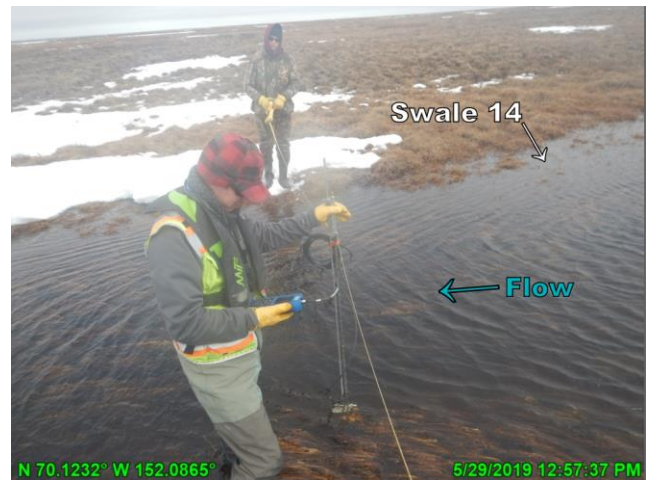
Photo 4.98: Measuring discharge near SW14, looking south (upstream); May 29, 2019
