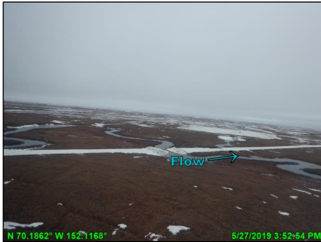
Photo 4.24: Slotted ice road near UC2C; looking southeast (upstream); May 27, 2019
