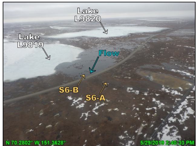
Photo F.16: Differential ponding near S6, looking southwest; May 29, 2019
