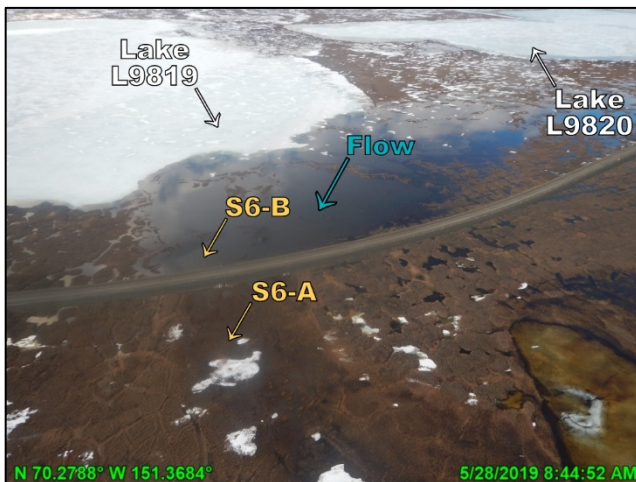
Photo 3.2: Local ponding on south side of GMT1/MT6 access road at site S6, looking south; May 28, 2019
