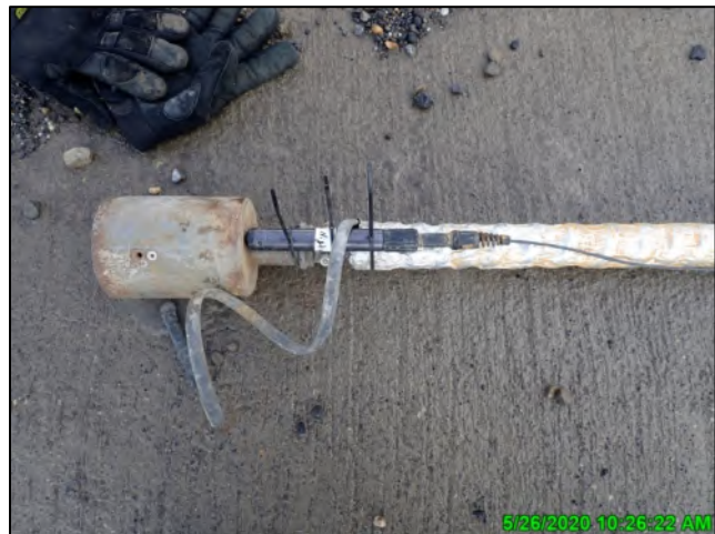
Photo 2-13: Pier scour sonar equipment on the Nigliagvik; May 26, 2020
