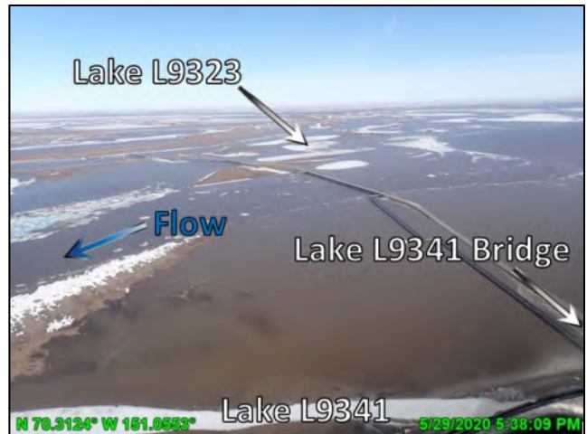
Photo 4-56: Overbank flooding near the Lake L9341 bridge crossing, looking southeast (upstream); May 29, 2020
