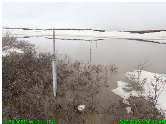
Photo 2-4: Indirect-read gages at G38; May 27, 2020
