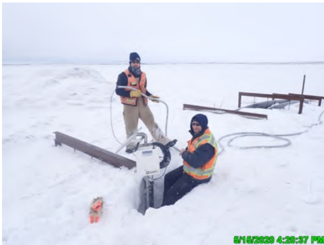
Photo 2-12: Remote stage monitoring equipment at Lake L9313 (G10); May 15, 2020
