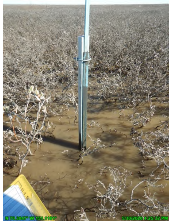
Photo 2-5: Observing and recording a high water mark on gage G38-C; May 30, 2020
