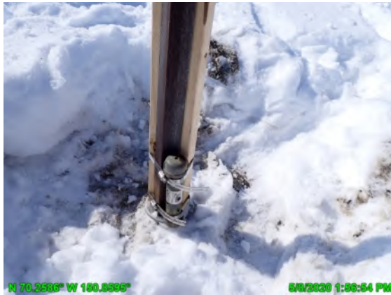
Photo 2-6: Installation of PT on staff gage MON9D-A; May 8, 2020
