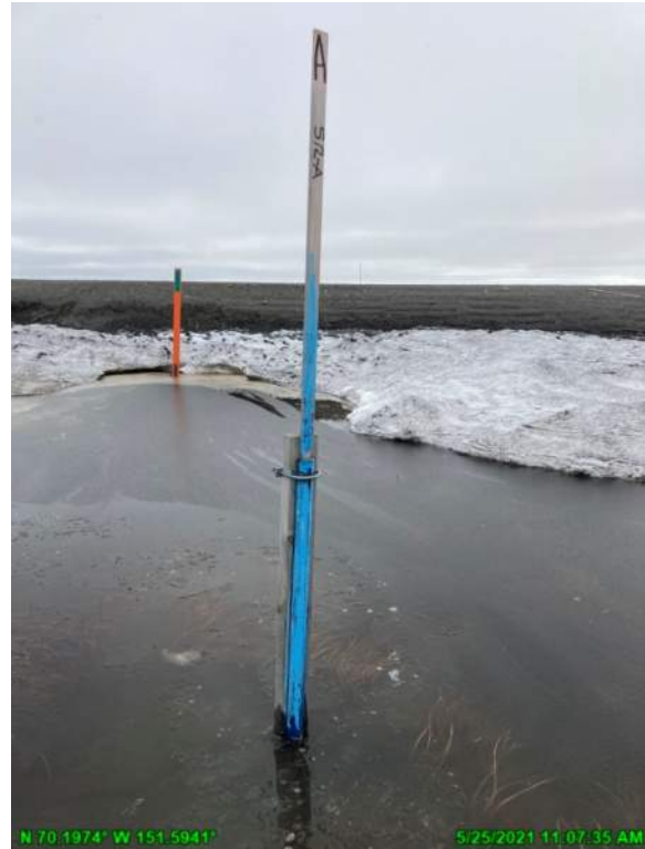
Photo 2.5: Observing and recording a high-water mark on gage S12-A; May 25, 2021
