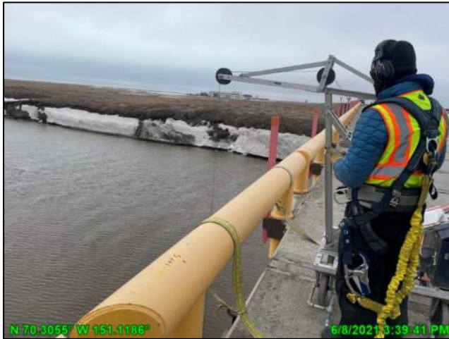
Photo 2.8: Measuring discharge at the Nigliagvik Bridge; June 8, 2021
