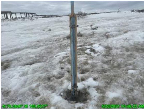
Photo 2.6: Installation of PT on staff gage SAK-A May 23, 2021
