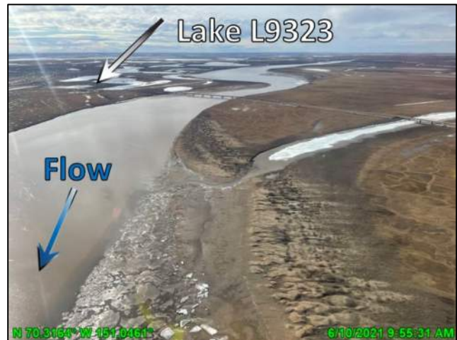
Photo 4.45: Lake L9323 bridge 3 days after peak stage showing no hydraulic connection, looking south; June 10, 2021
