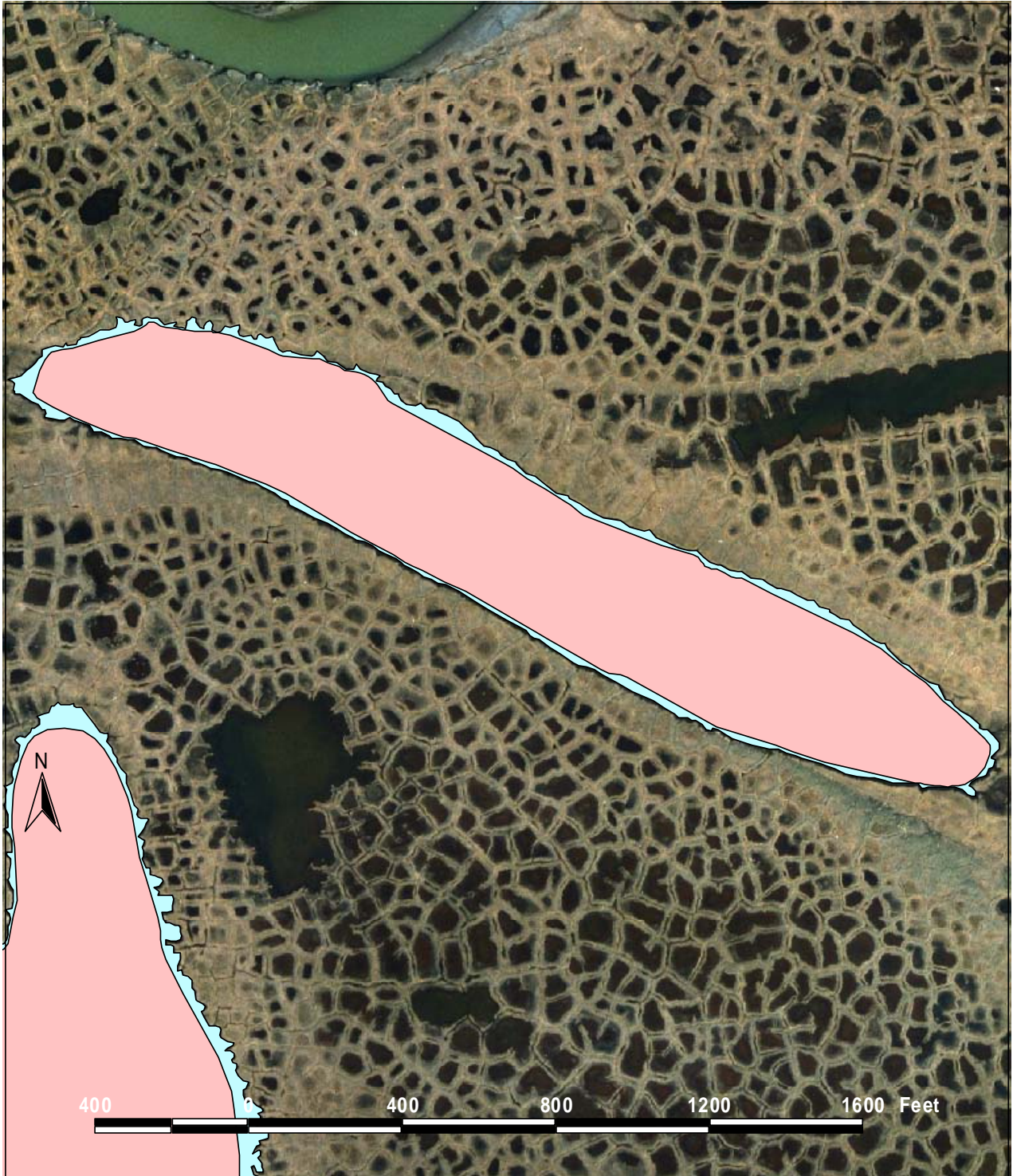
Regions of lake M9321 less than 4 feet deep (light shaded) and likely to be available for ice chips, based on transects surveyed on July 14, 2006.
