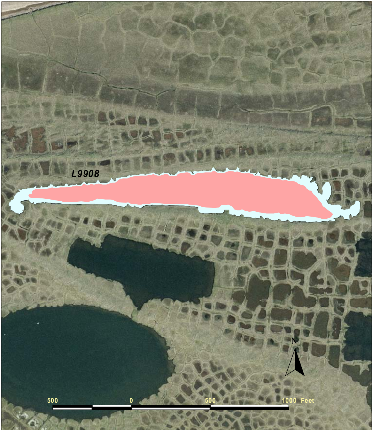
Regions of lake L9908 less than 4 feet deep (light shaded) and likely to be available for ice chips, based on transects surveyed on July 29, 2006.
