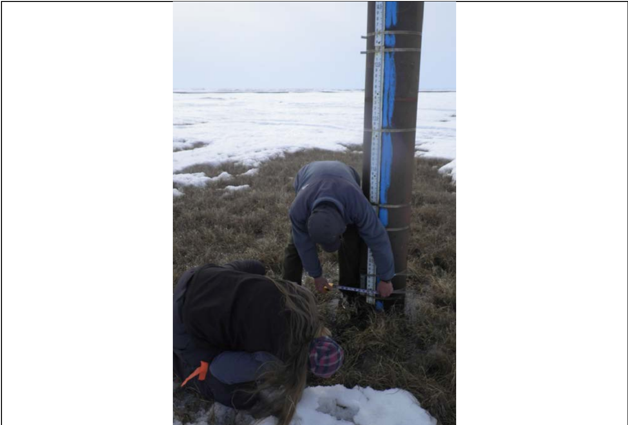
Photo 3: Installing pressure transducer at G11 near CD3 pad; May 12, 2014
