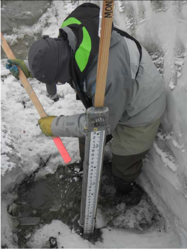
Photo 1: Chipping ice off gage; May 31, 2014
