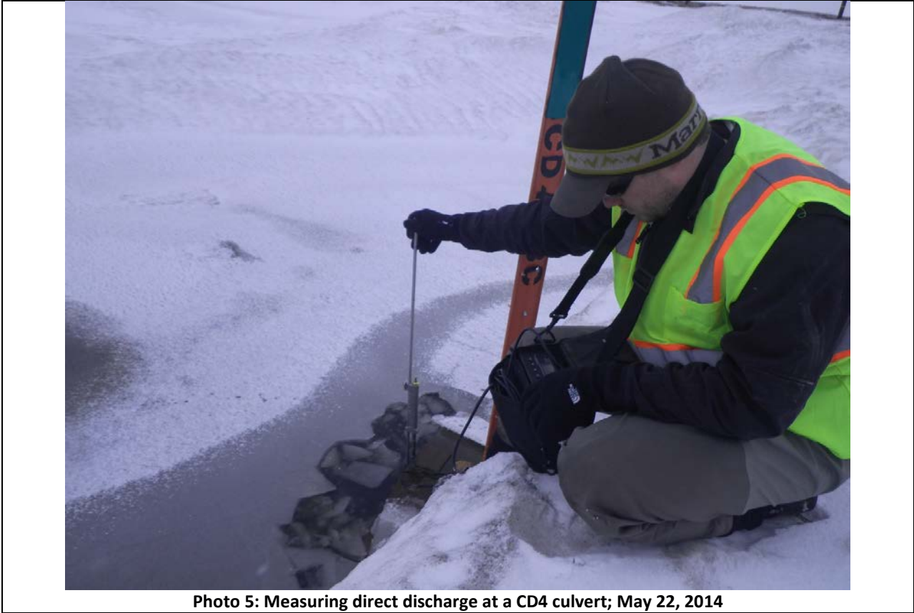
Photo 5: Measuring direct discharge at a CD4 culvert; May 22, 2014
