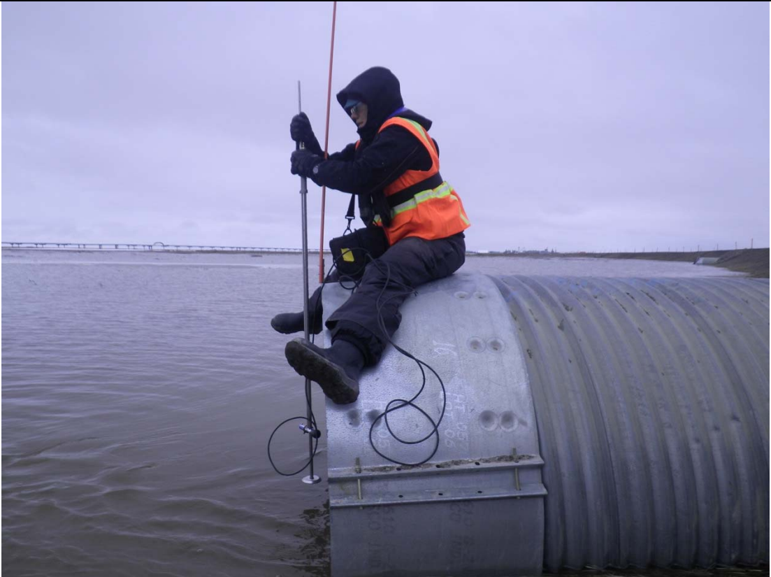
Photo 5: Collecting discharge measurements at a culvert along the CD2 road; June 2, 2014
