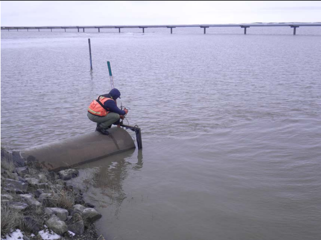
Photo 4: Collecting discharge measurements at a culvert along the CD2 road; June 2, 2014
