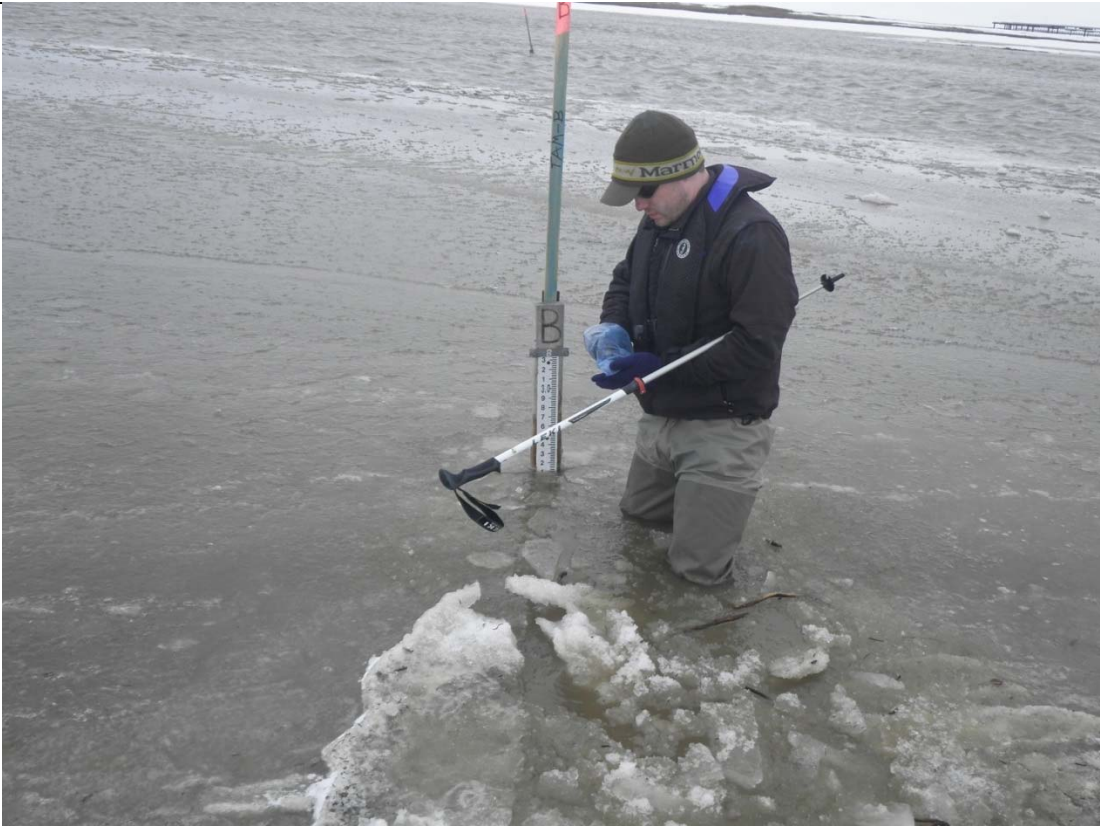
Photo 4: Re-chalking gage at Tamayayak Channel near the pipe bridge crossing; May 21, 2014
