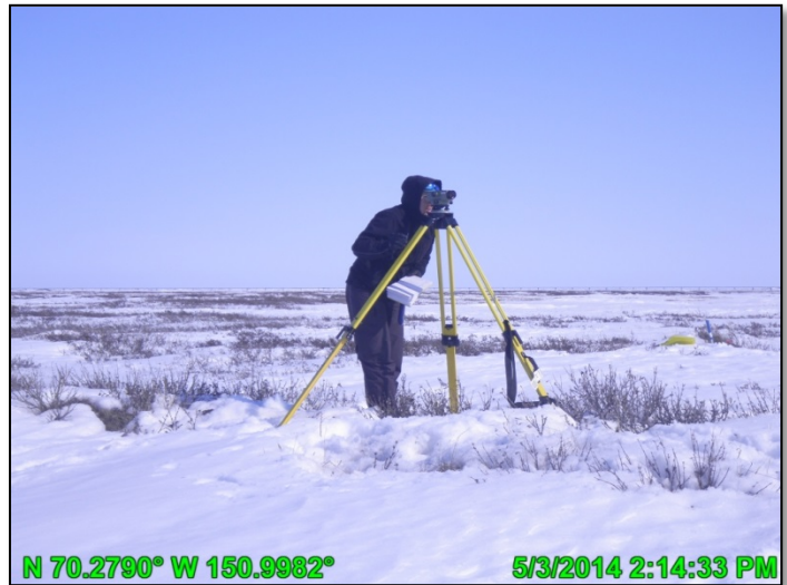
Photo 1: Conducting elevation surveys during spring breakup setup; May 3, 2014
