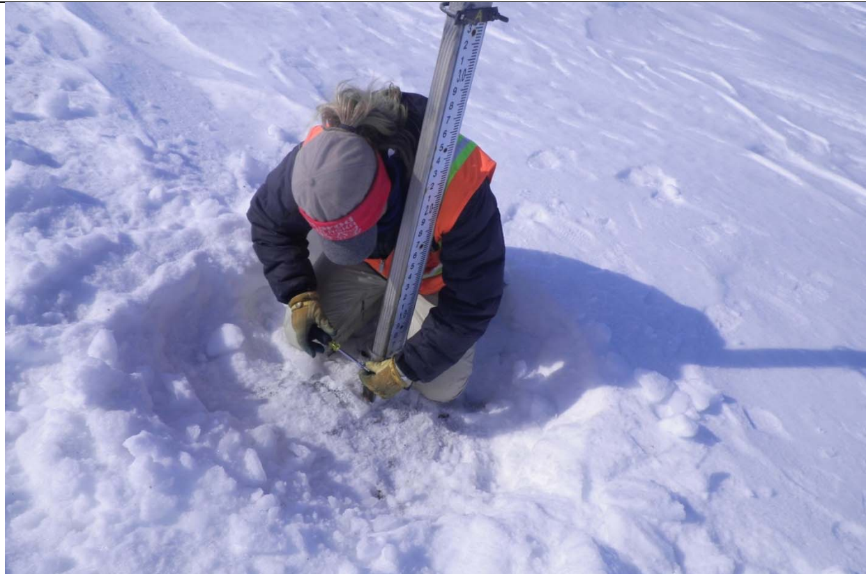
Photo 1: Installing a pressure transducer at MON28; May 6, 2014
