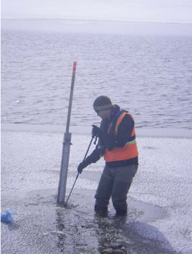
Photo 4: Gage reading and chalking at Lake M9525; May 23, 2014
