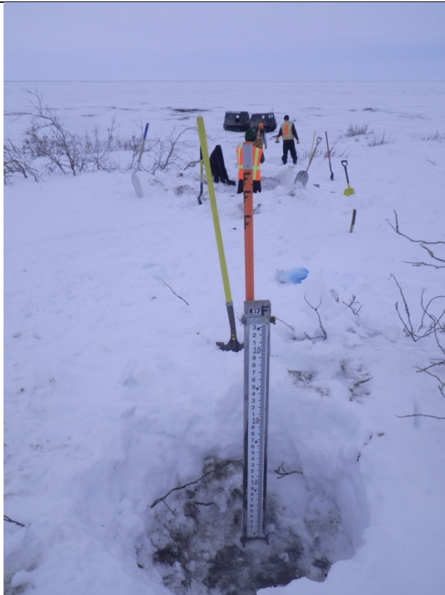
Photo 4: Field personnel rehabbing gages at MON1; May 1, 2014
