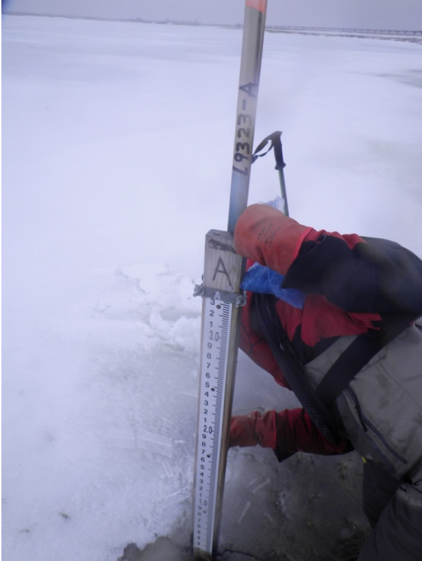
Photo 2: Chalking gage at Lake L9323; June 1, 2014
