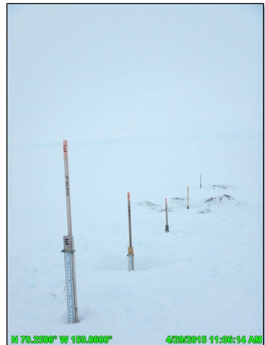
Photo 2.1: Gage set MON9D showing staff gage elevation overlap from the “A” gage nearest the channel to the “E” gage at the top of the bank; April 29, 2015
