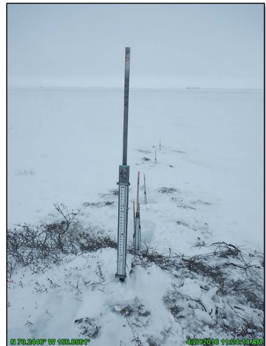
Photo 2.1: Gage set MON9 showing staff gage elevation overlap from the “A” gage nearest the channel to the “G” gage at the top of the bank; April 27, 2016
