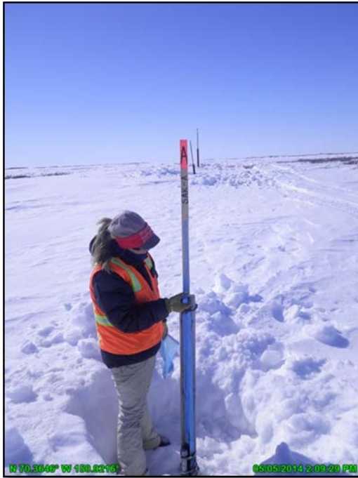
Photo 1.2: Setting up and chalking gages at the Sakoonang Channel adjacent to the pipeline bridge, looking southwest; May 5, 2014
