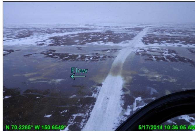
Photo C.17: Flow over the No Name Creek ice road crossing, looking northeast; May 17, 2014
