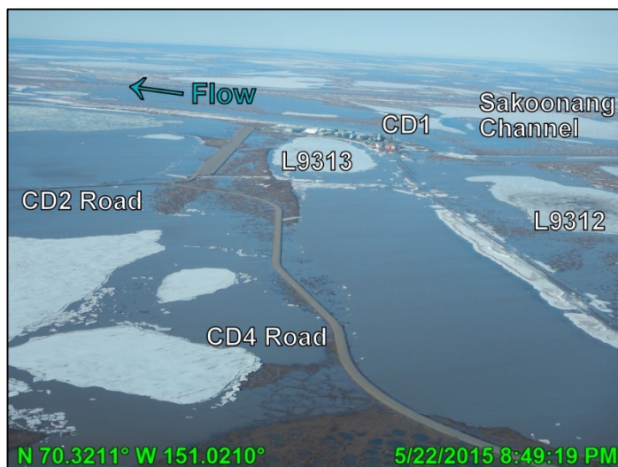
Photo 3.12: Inundation around CD1 showing hydraulic connection between the Sakoonang Channel and the drinking water source lakes, looking northeast following peak stage; May 22, 2015
