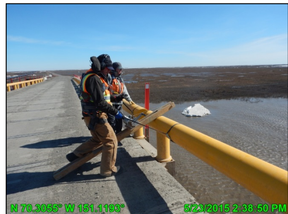
Photo 2.8: Discharge Measurements at the Nigliagvik Bridge; May 23, 2015
