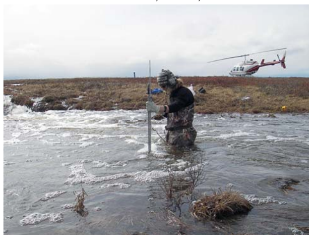
Photo 2-2 Small Stream Wading Discharge Measurement, June 7, 2006
