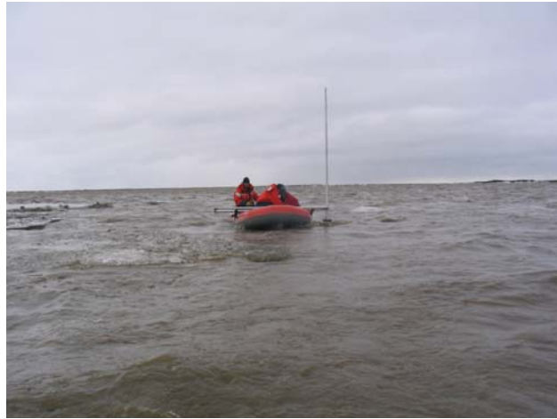
Photo 4-12 Direct Discharge (ADCP) Measurement on Colville River, May 29, 2006.
