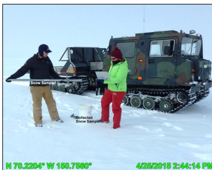
Photo 3.2: Collecting core using Mt. Rose Snow Sampler (Model 3600); April 25, 2015
