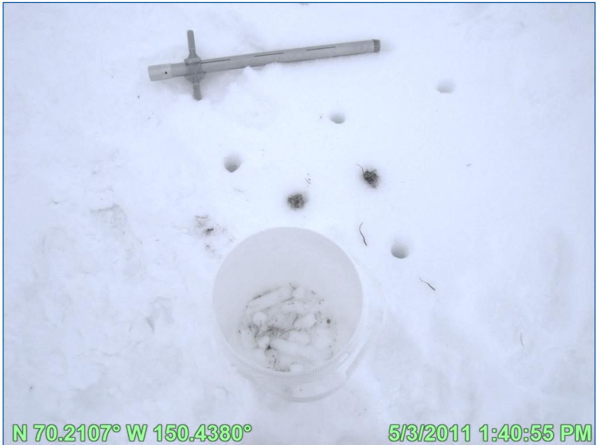
Photo 3.2: Model 360 Mt. Rose Snow Sampler (top) and bucket with pooled snow samples (bottom) with sample holes (2011 file photo); May 3, 2011
