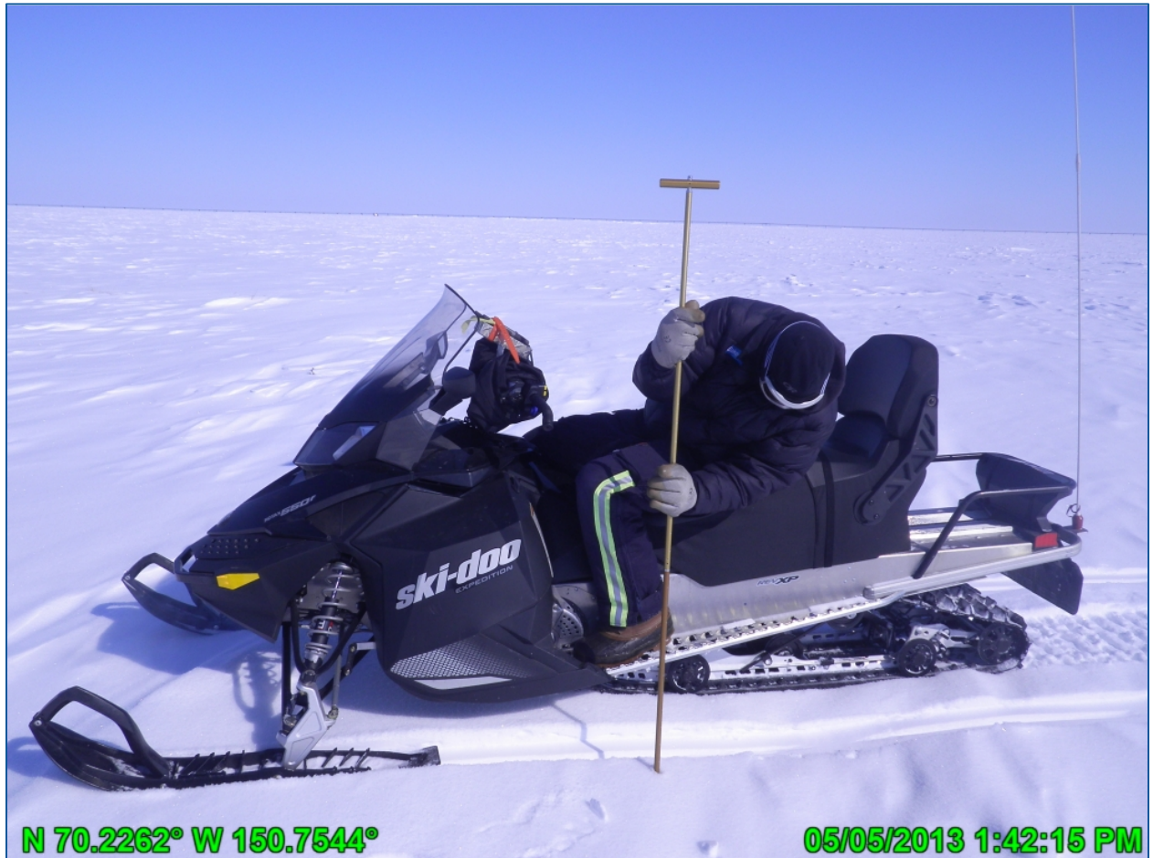
Photo 3.4: Field crew taking snow depth measurements with a graduated snow pole; May 5, 2013
