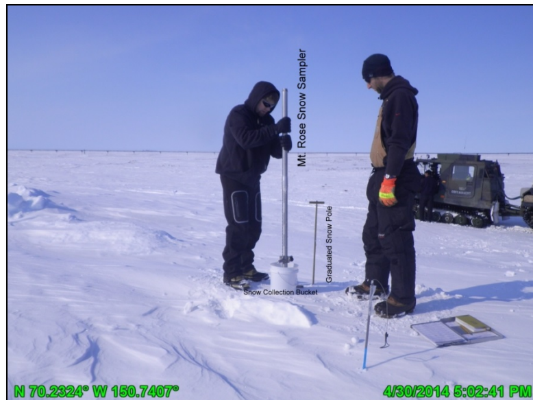
Photo 4: Field crew taking snow core with Mt Rose Sampler and depth measurements with a graduated snow pole; April 30, 2014
