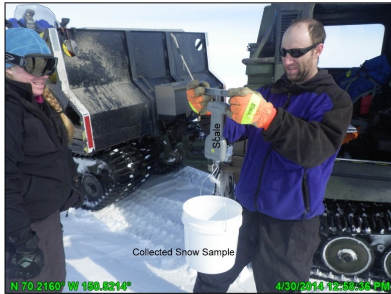
Photo 3: Weighing bucket of pooled snow samples; April 30, 2014
