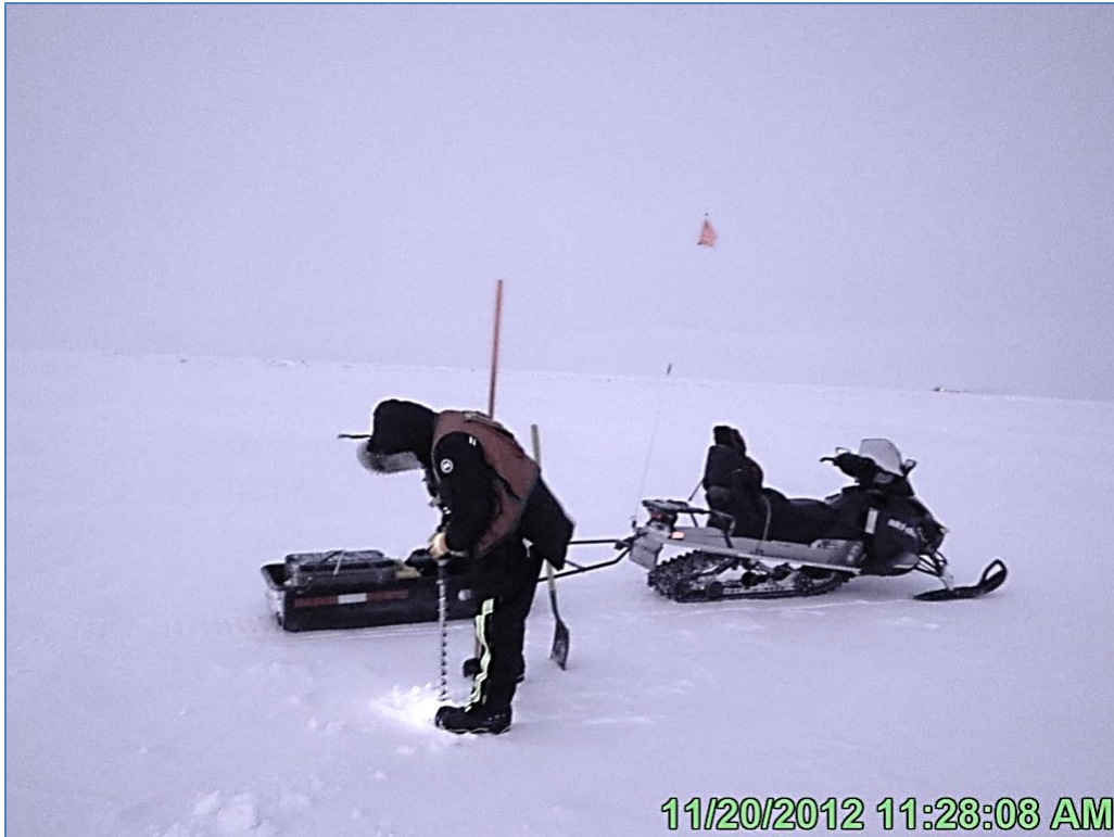
Photo B.5: Drilling hole using ice auger; November 20, 2012
