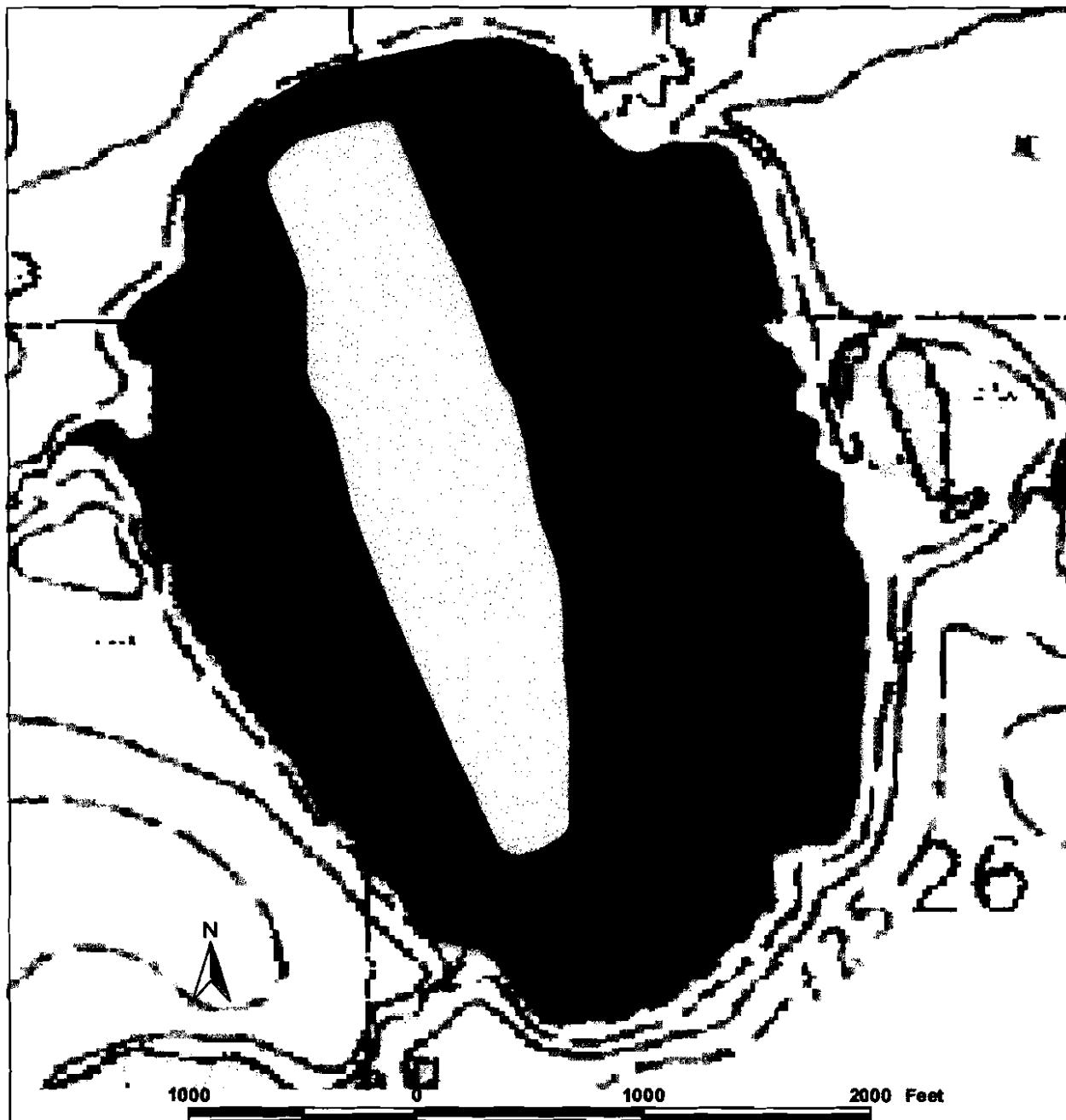
Regions of lake M0328 less than 4 ft deep (dark shaded), and likely to be available for ice chips, based on transects surveyed on August 1, 2003.
