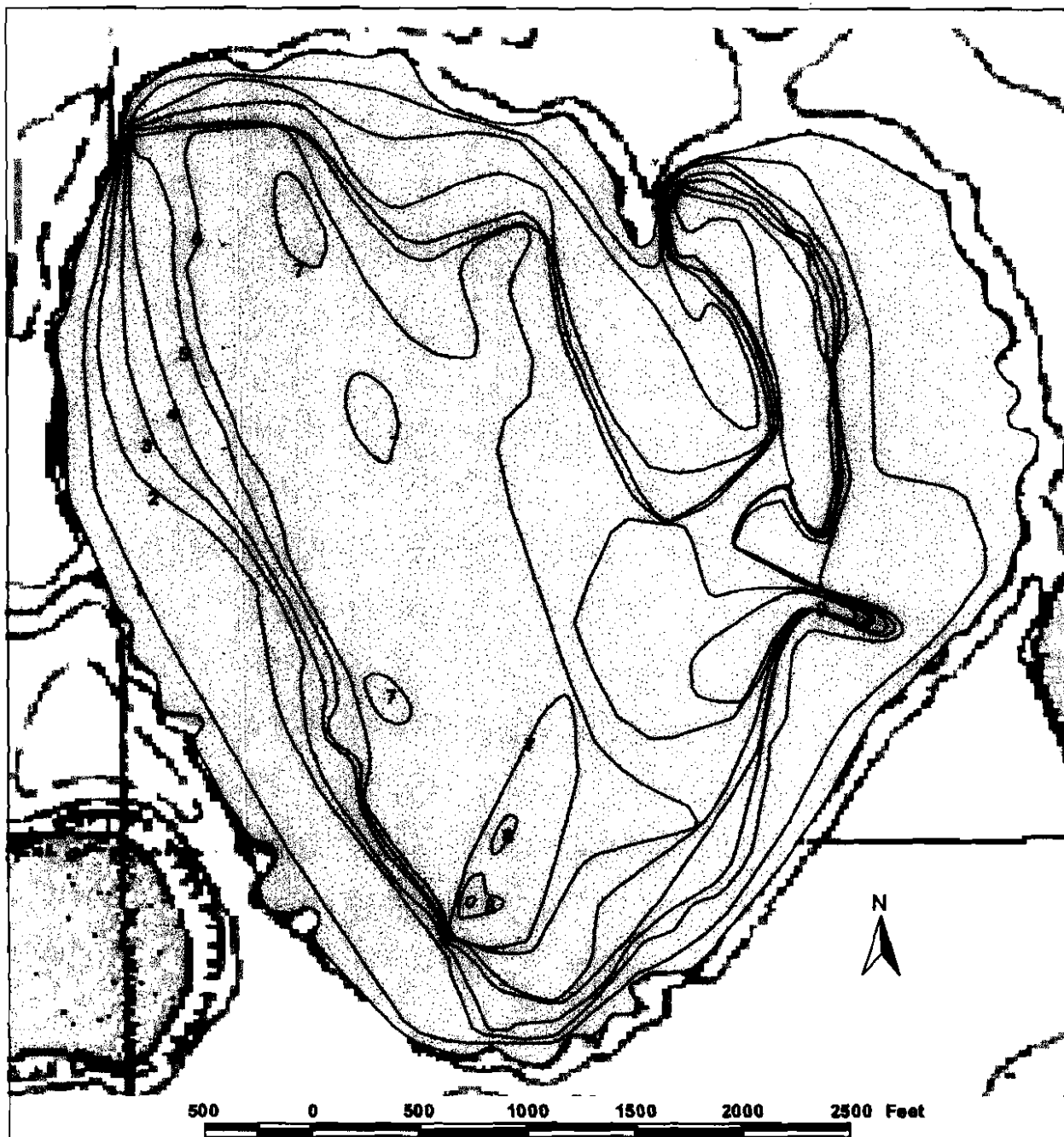
Depth contours of lake M0301, based on transects surveyed on July 12, 2003 (depth intervals in 1 foot increments)
