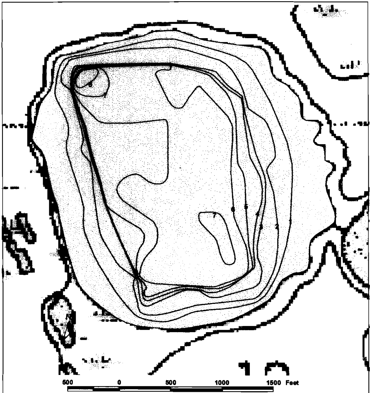
Depth contours of lake M0315, based on transects surveyed on July 19, 2003 (depth intervals in 1 foot increments)
