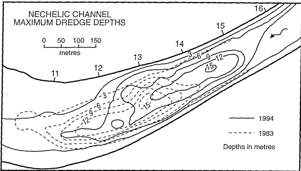
Figure 6. Map showing the shift upstream of dredging operations between 1983 and 1994
