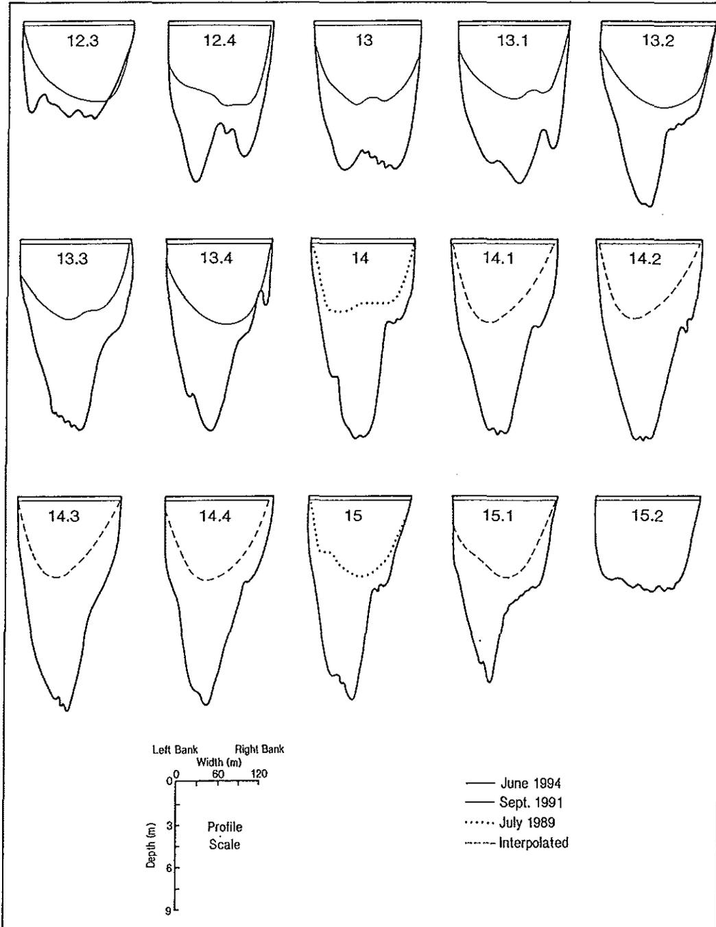
Figure 5. Cross-section surveys of 1992-1993 dredge channel
