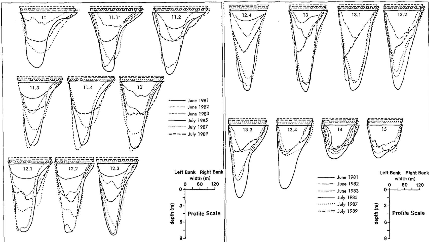
Figure 3. Cross-section surveys of the Nechelic dredge channel
