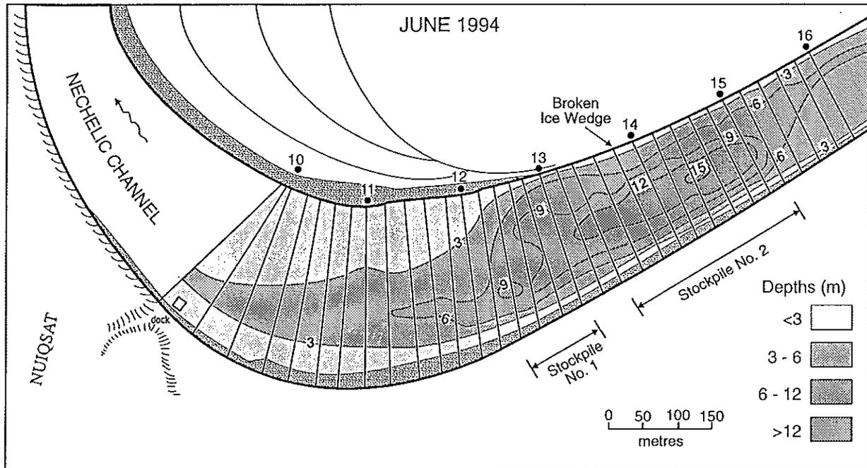
Figure 4. Dredge channel in June 1994
