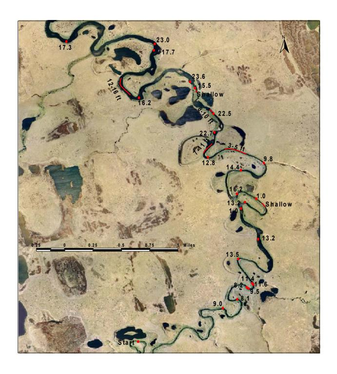
Figure 1. Depths (in feet) observed in the lower Ublutuoch River on July 30-31, 1999 during surveys conducted to identify potential ice road crossings (MJM Research data files).
