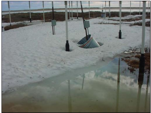
Photo 11 – HDD crossing, east bank. Uneven settling of protective CMP at thermistor string. June 17, 2004.
