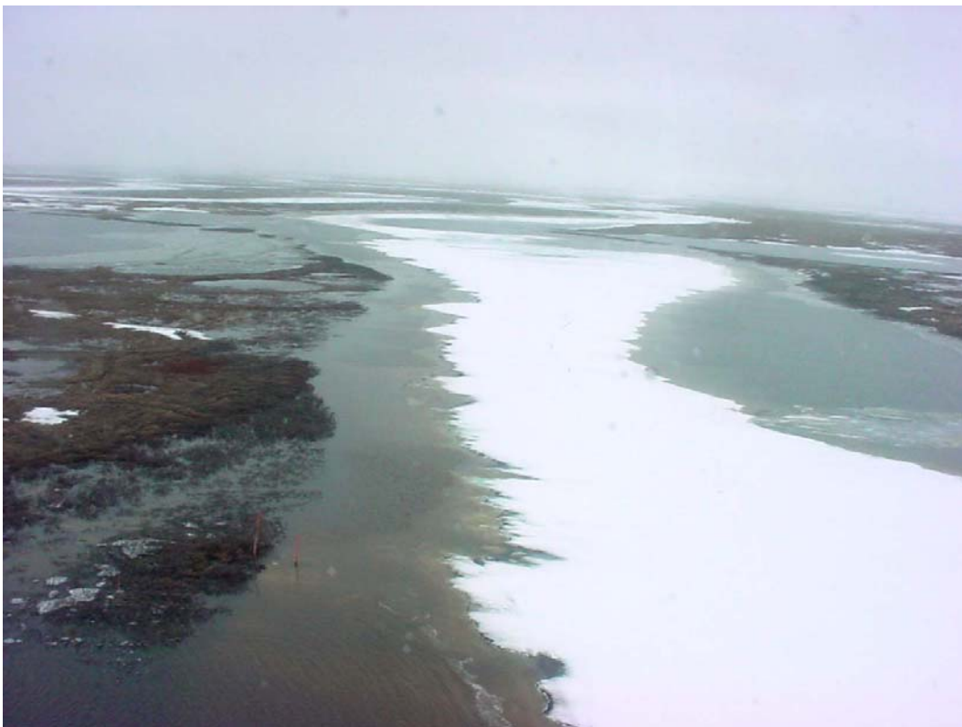
Photo 4-6 The water in the lower Ublutuoch River during the early stages of breakup was not flow from the Ublutuoch River itself, but rather backwater from flows over intact channel ice on Fish and Judy Creeks. Note that flooding from backwater extends to a point approximately one-quarter of a mile upstream of the gages (visible at lower left) at the Ublutuoch mile 1.9 monitoring site. May 30, 2004.
