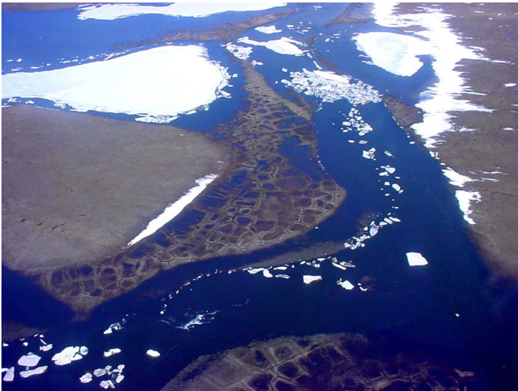
Photo 4-10 Water levels at the Ublutuoch bridge site (shown) dropped relatively quickly after the peak stage though small ice jams continued to cause localized, temporary water surface elevation increases that were reflected as secondary peaks on the hydrograph. June 9, 2004.
