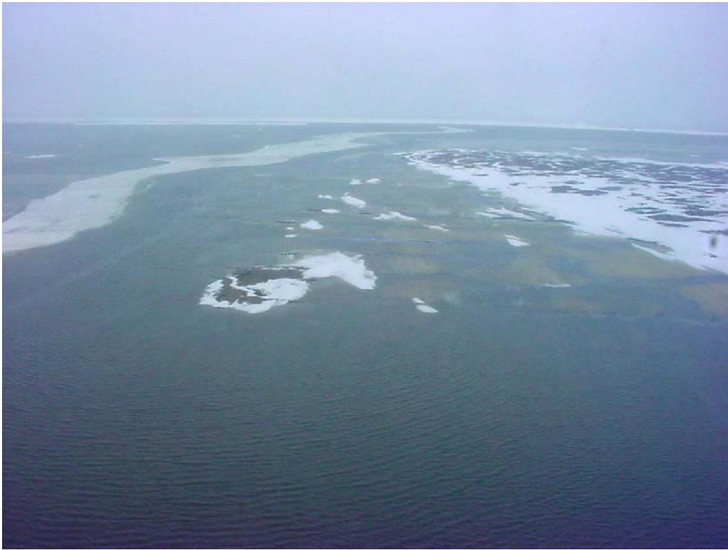
Photo 4-3 The relatively early occurrence of the peak stage at Fish 0.7 was likely a result of backwater effect from peaking floodwaters at the mouth of the Colville River combined with high wind. Note wind-driven southerly swell. May 30, 2004.
