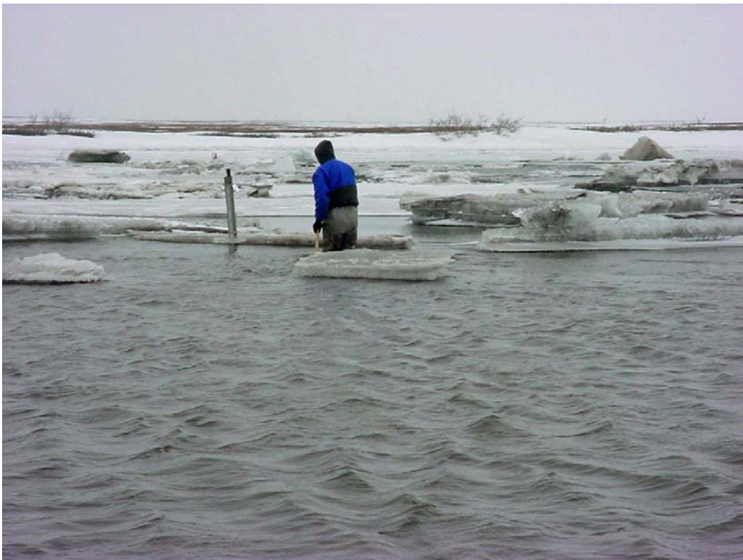
Photo 4-2 Breakup flooding on Fish Creek was characterized by heavy floating ice and frequent ice jamming that affected localized water surface elevations at some monitoring stations. May 30, 2004.
